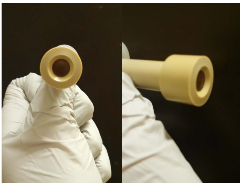
Figure S5. Electrode screw cap modified to eliminate effect of gas bubbles on the measured potential.
