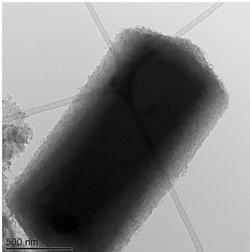
**Figure S6.** TEM of the unfunctionalized MCM-41 silica used as the catalyst support in all experiments.
