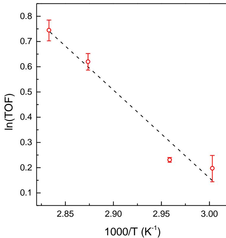
**Figure S3.** Arrhenius plot for the aldol condensation of 4-nitrobenzaldehyde with acetone from 60-80 °C using catalyst MCM-C4-0.57-A-HMDS with trimethylsilyl-capped silanols.
