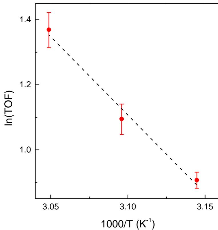
**Figure S2.** Arrhenius plot for the aldol condensation of 4-nitrobenzaldehyde with acetone from 45-55 °C using catalyst MCM-C4-0.57-A with available silanols.
