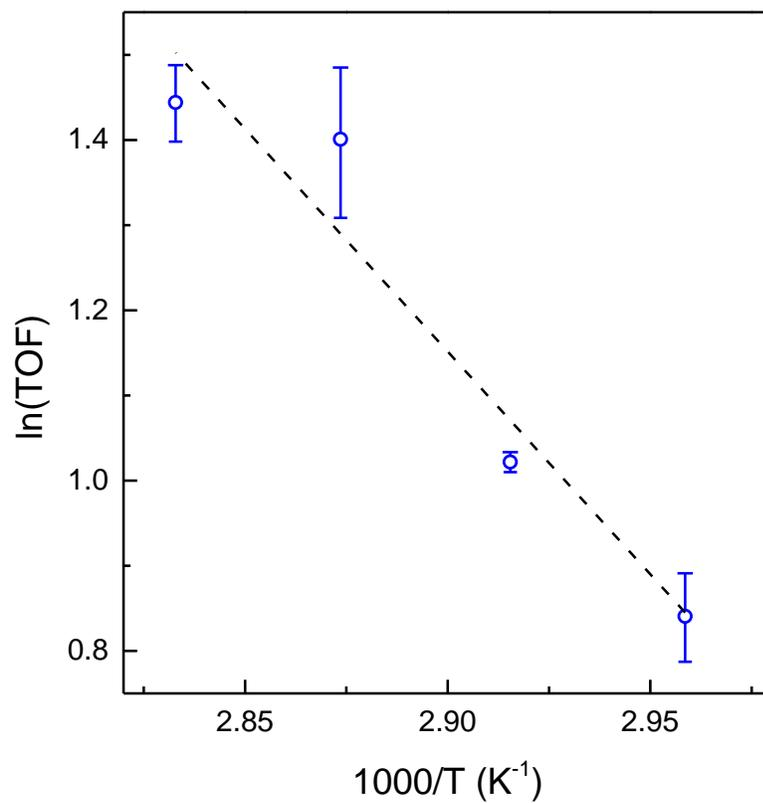
**Figure S5.** Arrhenius plot for the nitroaldol condensation of 4-nitrobenzaldehyde with nitromethane from 65-80 °C using catalyst MCM-C4-0.57-A-HMDS with trimethylsilyl-capped silanols.
