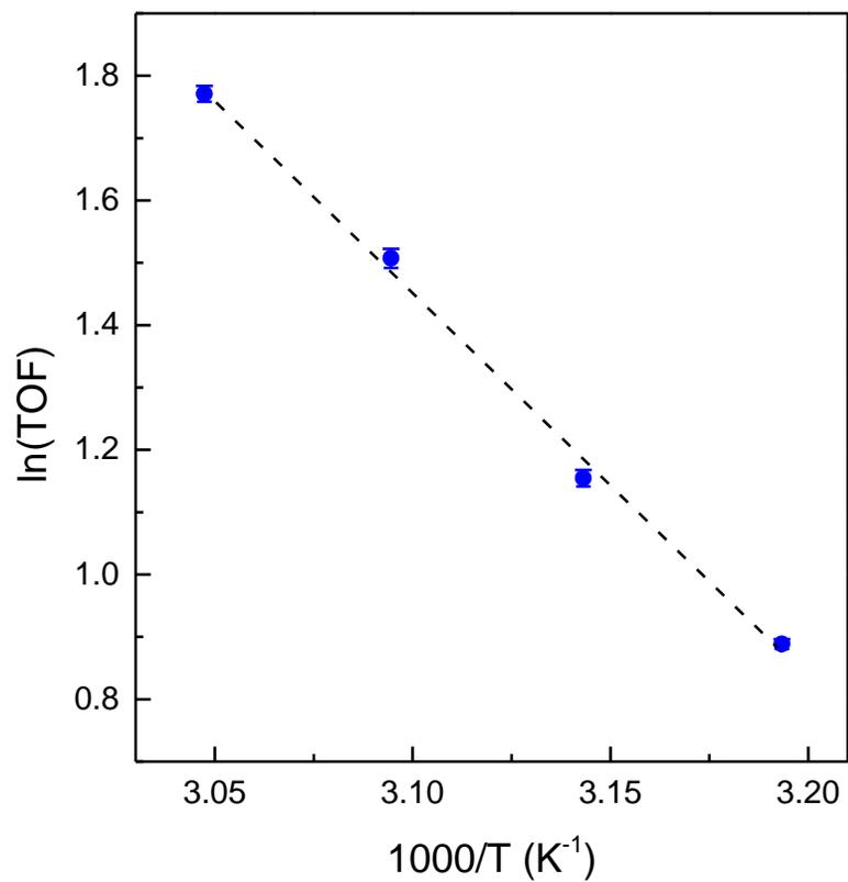
**Figure S4.** Arrhenius plot for the nitroaldol condensation of 4-nitrobenzaldehyde with nitromethane from 40-55 °C using catalyst MCM-C4-0.57-A with available silanols.
