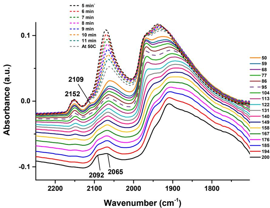
Figure S7 DRIFTS spectra taken during the temperature ramp to 200°C under helium after CO adsorption at room temperature.
