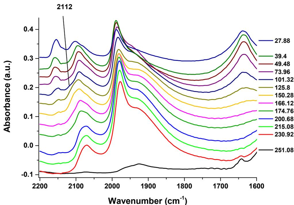
Figure S5 Selected DRIFTS spectra taken between 27-251°C during the CO oxidation experiment performed at the Pd K-edge.
