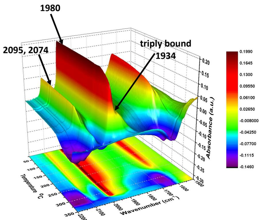
Figure S8 DRIFTS spectra recorded during the cooling step of the Pd K-edge experiment under CO oxidation conditions.
