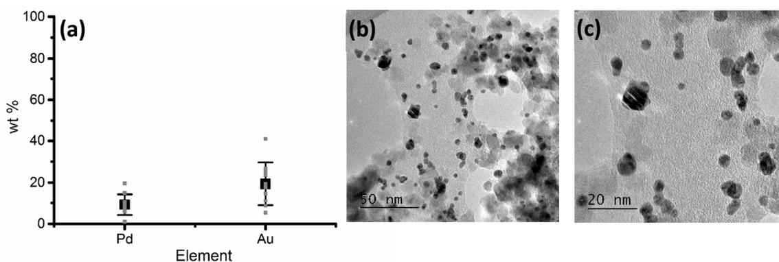
Figure S1 (a) The mean wt. % of Pd and Au (black squares), the standard deviation and the individual data for each particle (grey squares), representative TEM images of the AuPd/Al<sub>2</sub>O<sub>3</sub> catalyst at (b) 50 nm and (c) 20 nm resolution.
