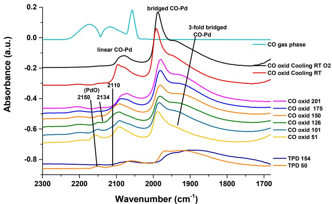
Figure S9 Selected DRIFTS spectra recorded during the CO TPD experiment, the reaction and cooling stages of the CO oxidation experiment and the CO gas phase spectrum.
