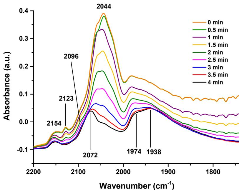
Figure S6 DRIFTS spectra taken during the helium purge after CO adsorption at room temperature.
