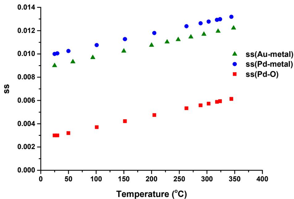
Figure S2 Change in the mean-squared relative displacement of absorber and backscatter atoms with temperature.
