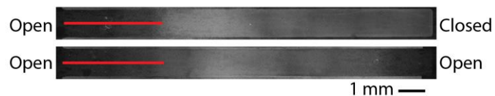
Fig S6. Comparison between plasma treated channels with one open (top) verse two open ends (bottom). Penetration distance of the channel with one open end is 3.67 mm and penetration distance into the channel with two open ends is 3.77 mm (penetration into the channel from the other end was not characterized).
