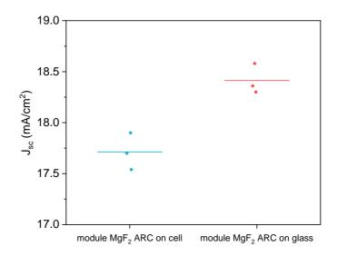
Figure S 1 The reverse-scan J<sub>sc</sub> summary of experimental modules.
