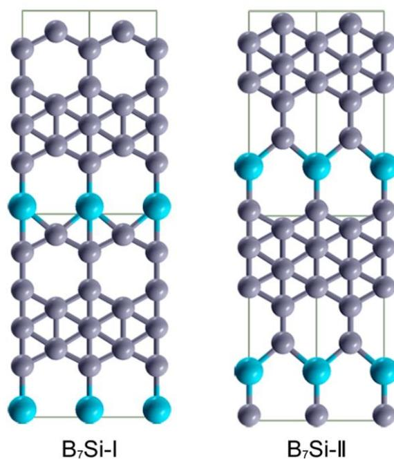
**Figure S8:** Low-energy monolayer structures of  $B_7Si$  from PSO search.
