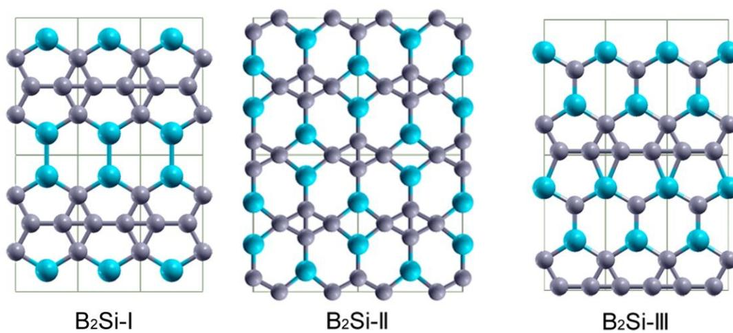
**Figure S4:** Low-energy monolayer structures of B<sub>2</sub>Si from PSO search.
