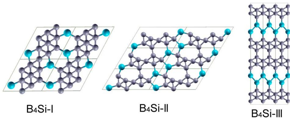
**Figure S5:** Low-energy monolayer structures of B<sub>4</sub>Si from PSO search.
