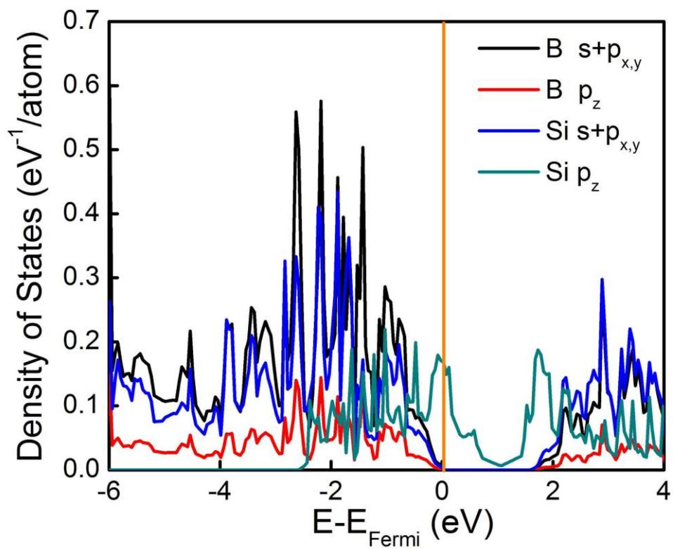
**Figure S9:** Partial density of states of 2D BSi<sub>4</sub>-I.
