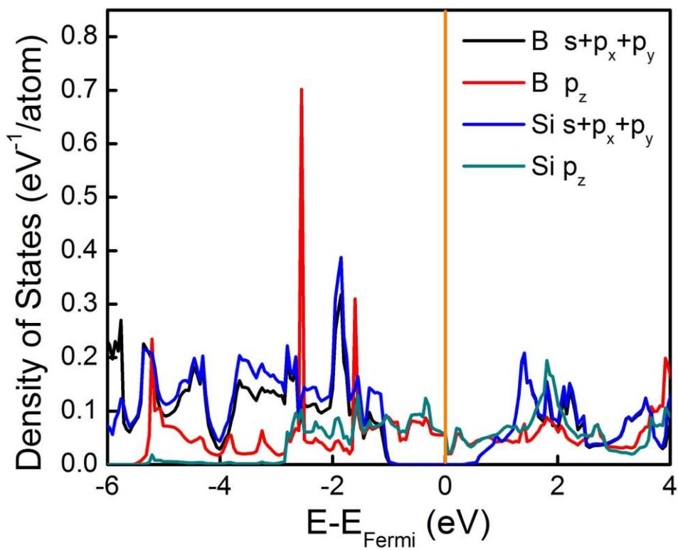
**Figure S10:** Partial density of states of 2D B<sub>3</sub>Si-I.
