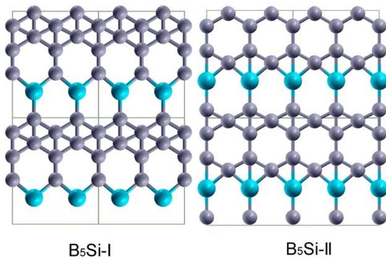
**Figure S6:** Low-energy monolayer structures of B<sub>5</sub>Si from PSO search.
