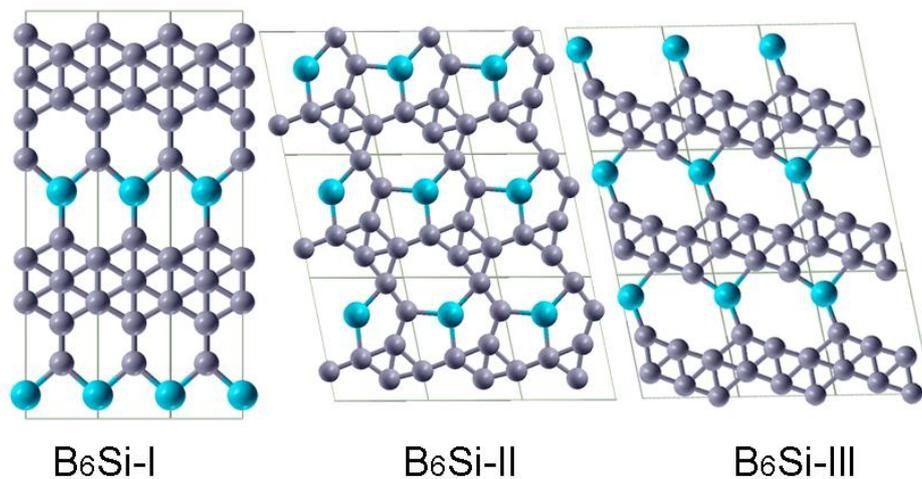
**Figure S7:** Low-energy monolayer structures of  $B_6Si$  from PSO search.
