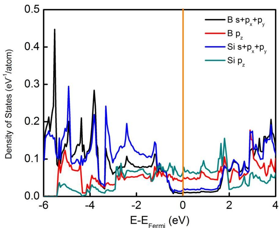
**Figure S11:** Partial density of states of 2D B<sub>4</sub>Si-I.
