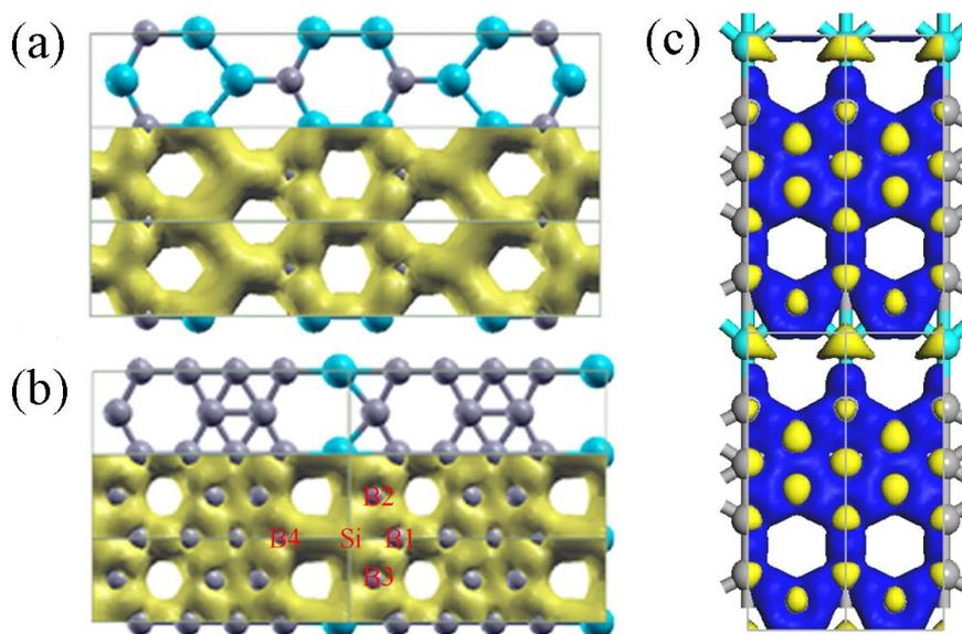
**Figure S12:** Computed iso-surfaces of electron localization function (ELC) with the value of 0.5 for (a) BSi<sub>2</sub>-I and (b) B<sub>7</sub>Si-I. (c) Iso-surface (0.05 e/au) of the computed deformation electron density for B<sub>7</sub>Si-I, where blue and yellow region refers to electron rich and deficient, respectively.
