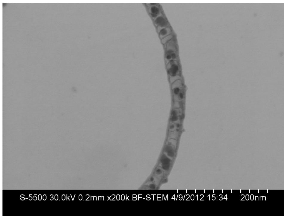
Figure S1. TEM image of N-CNT before acid treatment. Residual metal nanoparticles formed by the decomposition of ferrocene are observed.
