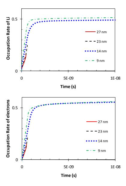
**Figure S1.** Grain size effect for  $\text{Li}^+$  and electron polaron transport in  $\text{TiO}_2$  grains with localized carbon coating and sizes 9, 14, 23 and 27 nm. The charge injection rate is  $2 \times 10^{10}$  per site per second.
