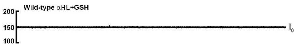
Figure S12. The single channel electric recordings based on wild-type \alpha HL nanopore in the presence of GSH. All nanopore experiments were carried out at +100 mV voltage.
