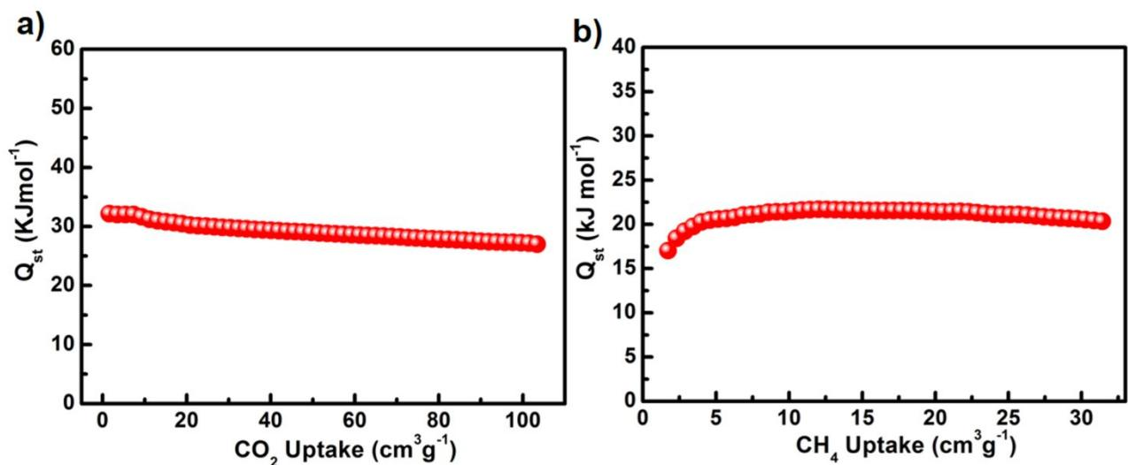
**Figure S20.**  $Q_{st}$  values calculated using the Clausius-Clapeyron equation of a)  $\text{CO}_2$  and b)  $\text{CH}_4$  for JLU-MOF107.
