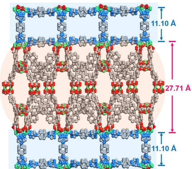
**Figure S4.** The distances between the unique layers.
