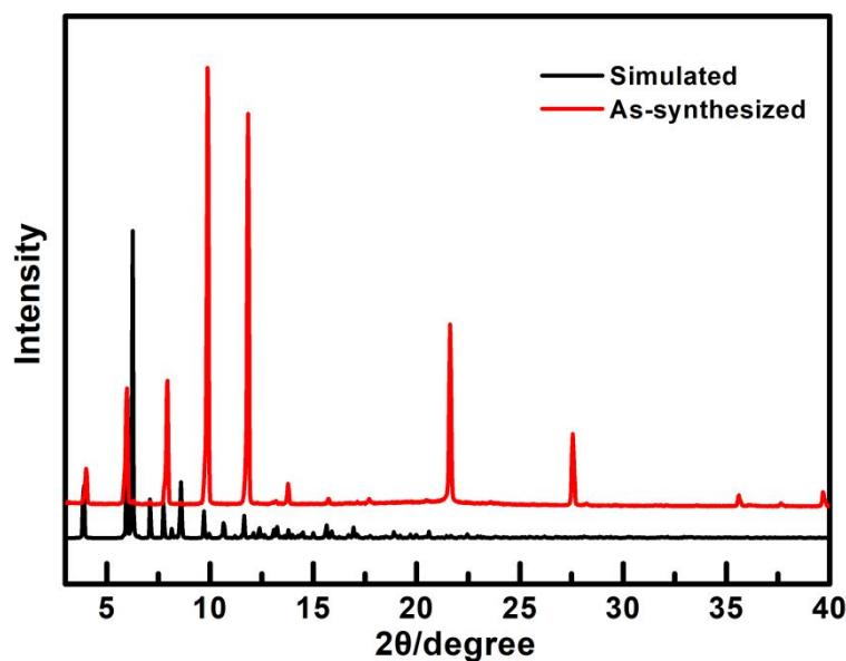
**Figure S14.** PXRD patterns of the simulated and as-synthesized JLU-MOF107.
