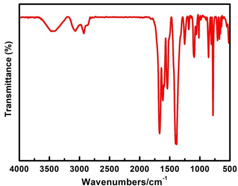
**Figure S12.** FT-IR spectrum of JLU-MOF107.
