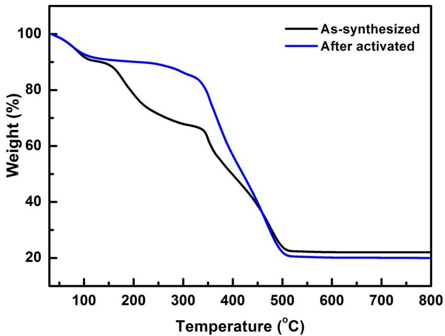
**Figure S18.** TGA curves of the as-synthesized and activated (acetonitrile exchanged) samples for JLU-MOF107.
