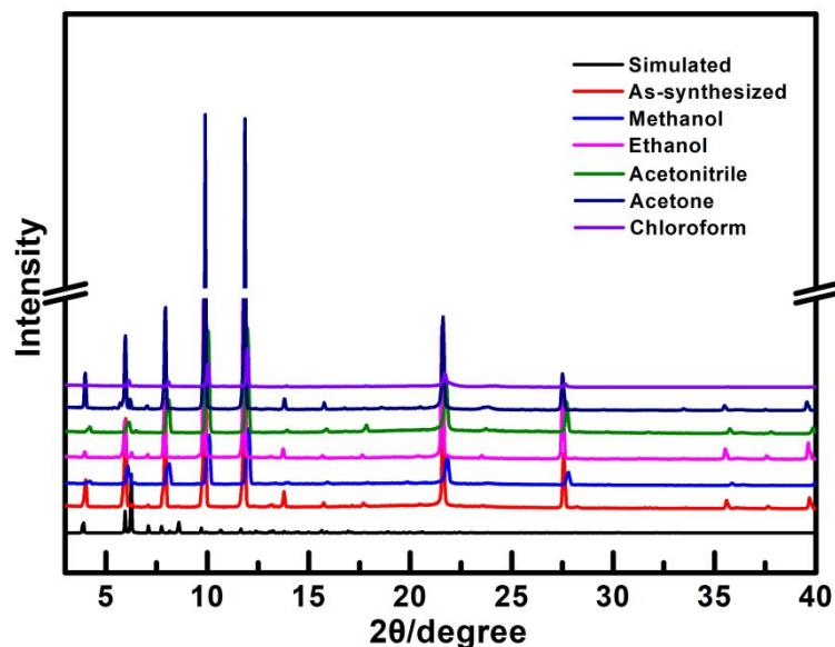
**Figure S15.** PXRD patterns of different solvent-exchanged JLU-MOF107 samples.
