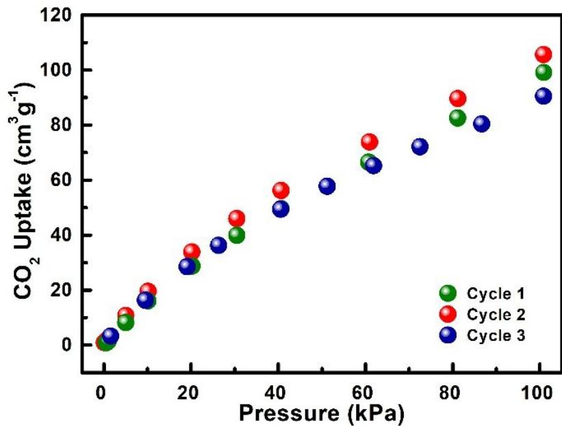
**Figure S23.** Three-cycle  $\text{CO}_2$  adsorption tests at 298 K for JLU-MOF107.
