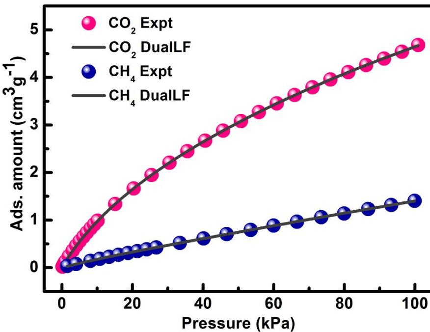
**Figure S22.**  $\text{CO}_2$  and  $\text{CH}_4$  isotherms at 298 K along with the dual-site Langmuir–Freundlich (DSLF) fits for JLU-MOF107.
