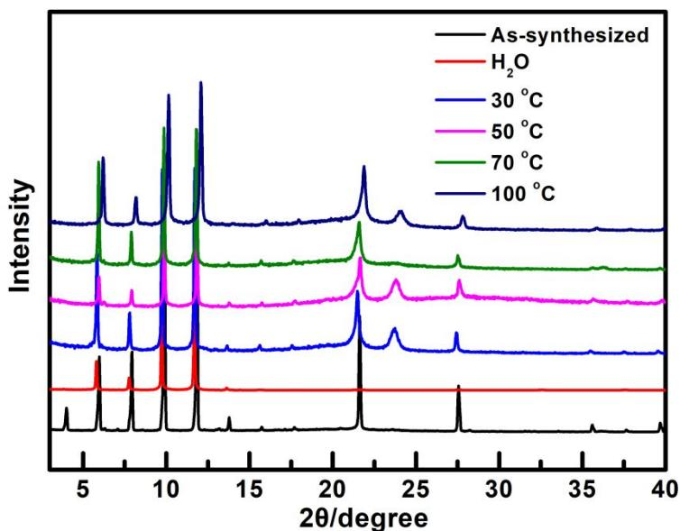
**Figure S17.** PXRD patterns of as-synthesized and immersed in water at different temperatures for JLU-MOF107.
