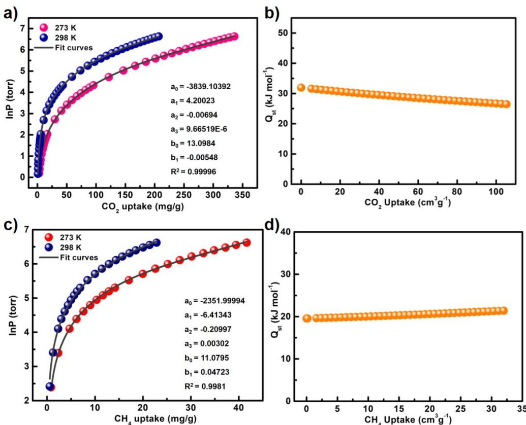
**Figure S21.** a) The fitting parameters of the virial model with the isotherms at 273 and 298 K for a)  $\text{CO}_2$  and c)  $\text{CH}_4$ ;  $Q_{st}$  values of b)  $\text{CO}_2$  and d)  $\text{CH}_4$ .
