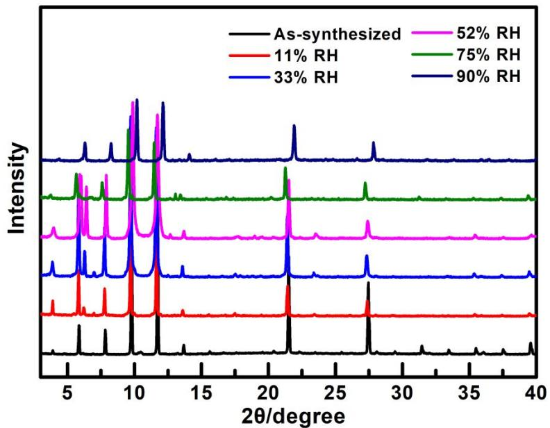
**Figure S16.** PXRD patterns of as-synthesized and exposed JLU-MOF107 under different relative humidity (RH) condition for 1 week.
