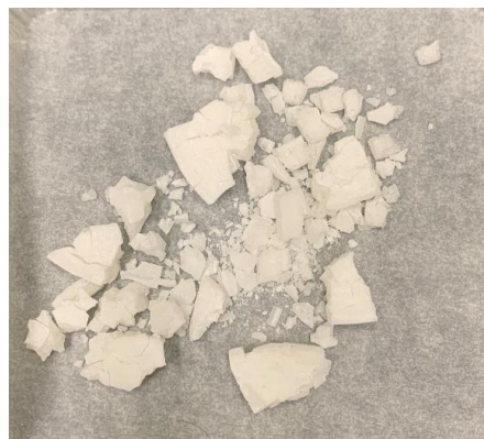
Brittleness and increased white color of N10 after 1 week in laboratory
