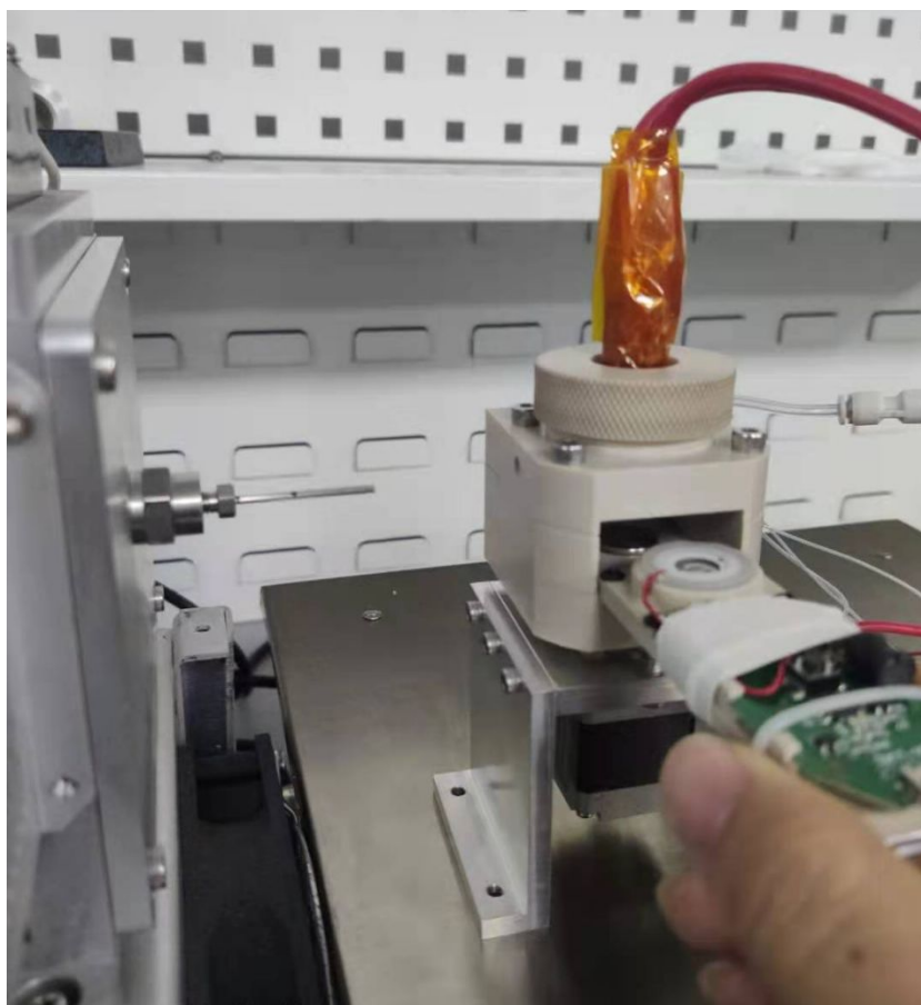
Figure S-2. Photograph of designed NSAP source
