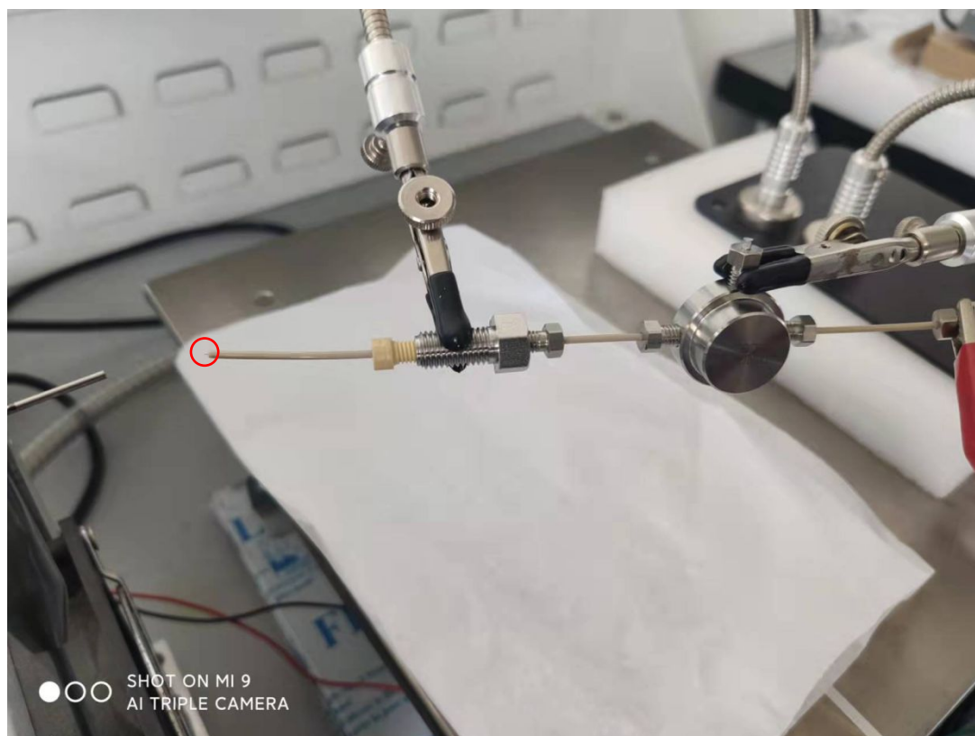
Figure S-3. Photograph of infusion ESI (10 \mu\text{L}/\text{min} )
