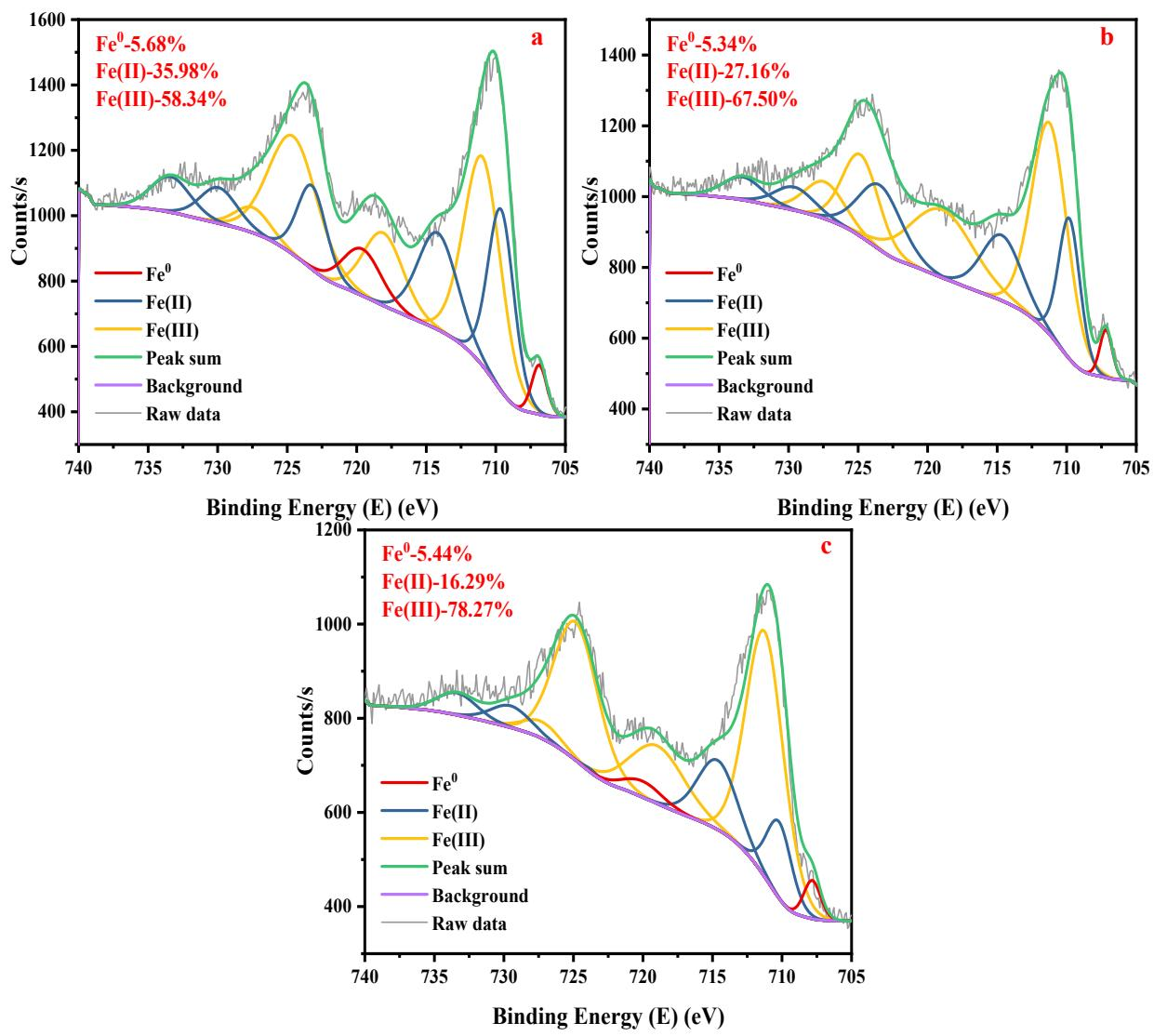
72 **Fig. S10.** XPS spectra of Fe 2p for the magnetically recovered nZVI<sub>100</sub> from (a) nZVI<sub>100</sub>, (b)
