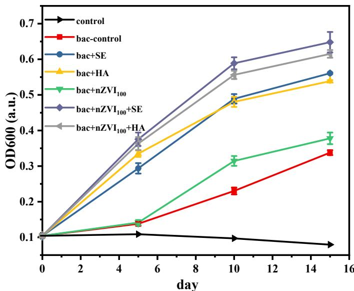
80 **Fig. S13.** Variation of microbial density in the mineral culture medium (PCP=10 mg/L) with nZVI<sub>100</sub>
