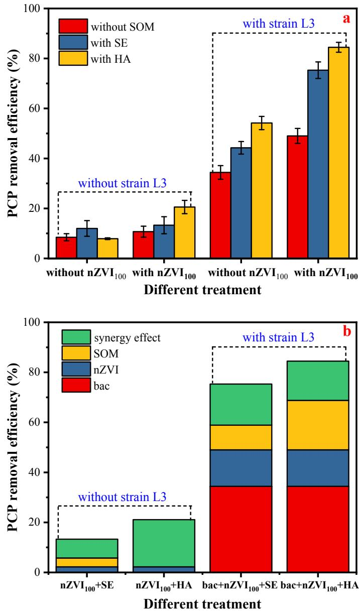
61 **Fig. S6.** (a) PCP removal efficiency and (b) contributions of bac, nZVI, and SOMs in different
