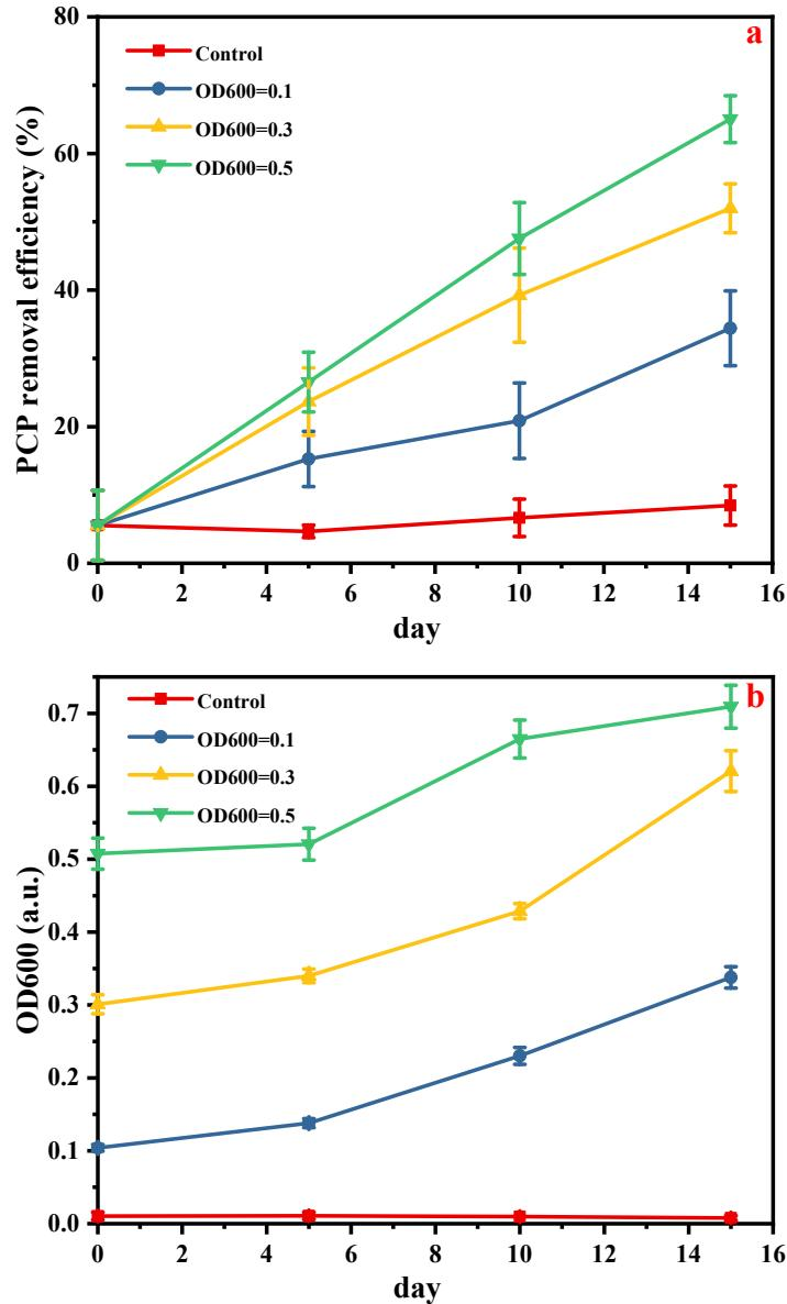
55 **Fig. S4.** Changes in (a) PCP removal efficiency and (b) bacterial density of reactors (PCP=10 mg/L)
