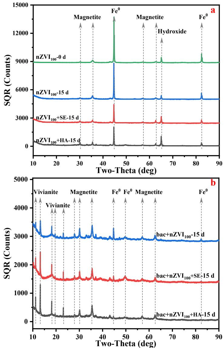
69 **Fig. S9.** XRD spectra of the pristine nZVI<sub>100</sub> and the magnetically recovered nZVI<sub>100</sub> after 15 day
