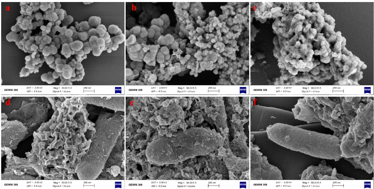
66 **Fig. S8.** SEM images of the magnetically recovered nZVI<sub>100</sub> for (a) nZVI<sub>100</sub>, (b) nZVI<sub>100</sub>+SE, (c)
