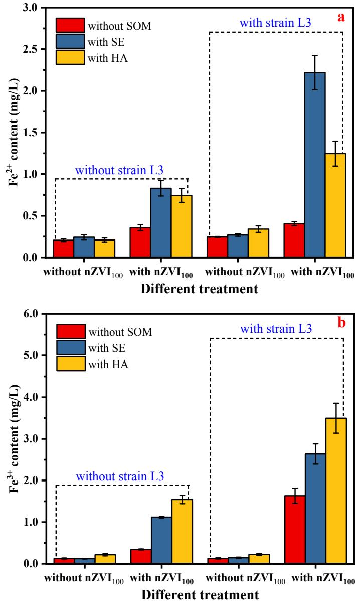
64 **Fig. S7.** Contents of (a)  $\text{Fe}^{2+}$  and (b)  $\text{Fe}^{3+}$  in sterilized and L3 strain reactors (PCP=10 mg/L) after 15
