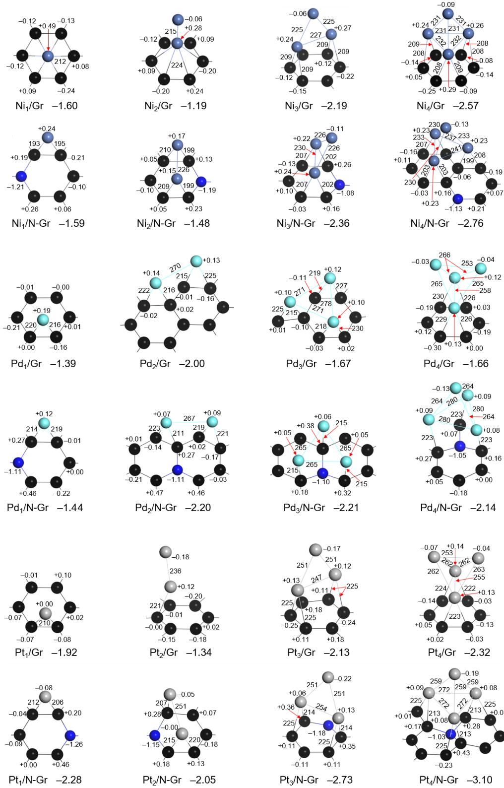
**Figure S4.** Bond lengths (pm),  $E_{\text{ads}}$  (eV), and Bader charges ( $e$ ) for the most stable configurations of TM<sub>n</sub> clusters (TM = Ni, Pd and Pt; n = 1–4) adsorption on Gr and N-Gr surfaces. Ni, Pd and Pt atoms are shown in blue, cyan, and grey balls, respectively.
