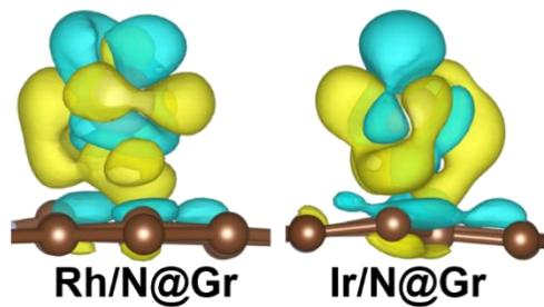
**Figure S24.** The main and side view of the 3D charge density difference plots for Rh<sub>1</sub>/N-Gr and Ir<sub>1</sub>/N-Gr, respectively, where the isosurface value is set to be 0.005  $e/\text{bohr}^3$ .
