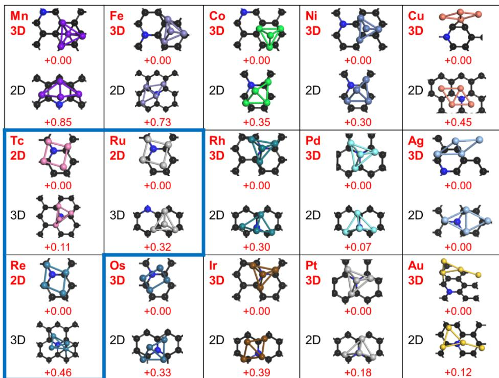
**Figure S26.** Comparison of 3D growth mode and 2D growth mode for tetramers on Gr and N-Gr surfaces with relative energies (eV).
