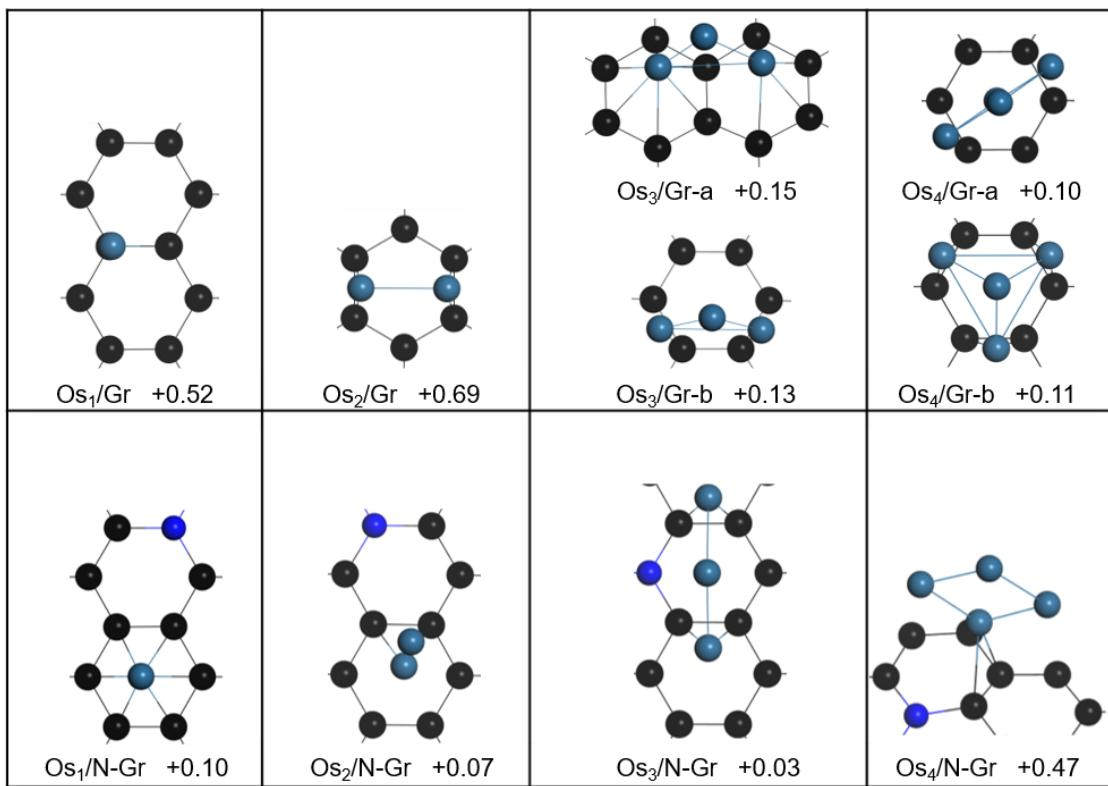
**Figure S11.** The sub-stable structures of Os<sub>n</sub> (n=1–4) adsorption on Gr and N-Gr surfaces with relative energies  $\Delta E$  (eV).
