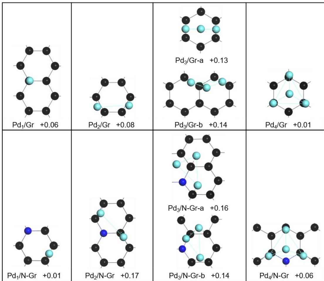
**Figure S16.** The sub-stable structures of Pd<sub>n</sub> (n=1–4) adsorption on Gr and N-Gr surfaces with relative energies  $\Delta E$  (eV).
