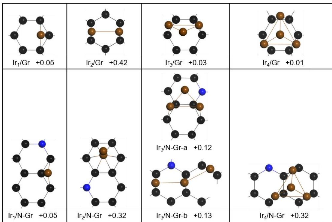
**Figure S14.** The sub-stable structures of  $\text{Ir}_n$  ( $n=1\text{--}4$ ) adsorption on Gr and N-Gr surfaces with relative energies  $\Delta E$  (eV).
