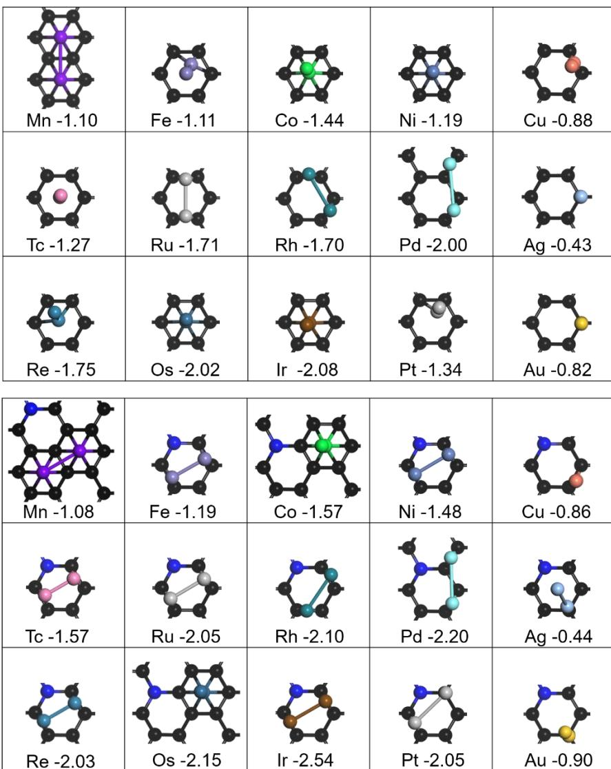
**Figure S21.** Summary for the adsorption of TM dimers on Gr (the top) and N-Gr (the bottom) surfaces with associated  $E_{\text{ads}}$  (eV).
