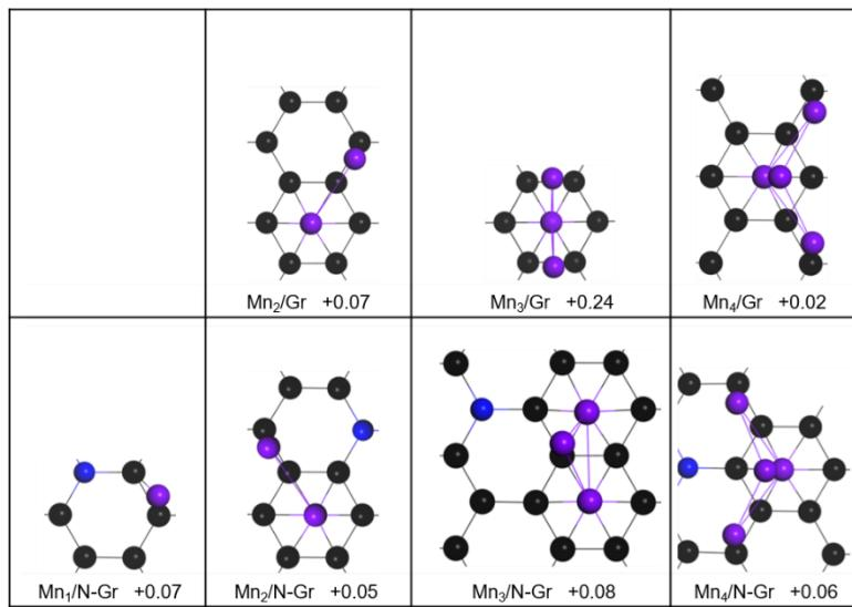
**Figure S6.** The sub-stable structures of Mn<sub>n</sub> (n=1–4) adsorption on Gr and N-Gr surfaces with relative energies  $\Delta E$  (eV).
