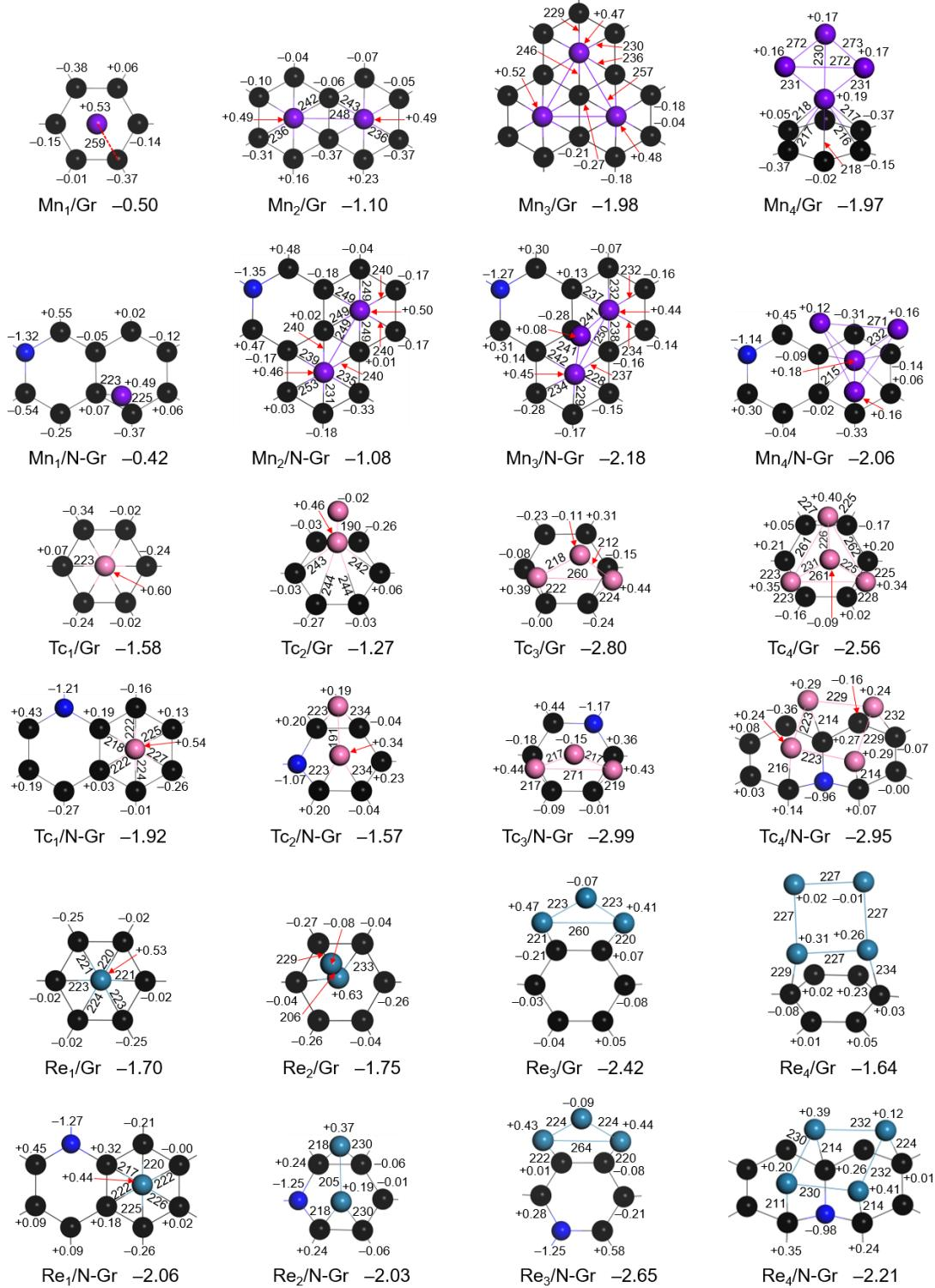
**Figure S1.** Bond lengths (pm),  $E_{\text{ads}}$  (eV), and Bader charges ( $e$ ) for the most stable configurations of  $\text{TM}_n$  clusters ( $\text{TM} = \text{Mn}, \text{Tc}$  and  $\text{Re}$ ;  $n = 1–4$ ) adsorption on Gr and N-Gr surfaces. Mn, Tc and Re atoms are shown in violet, pink, and green balls; C and N in black and deep blue balls for all figures.
