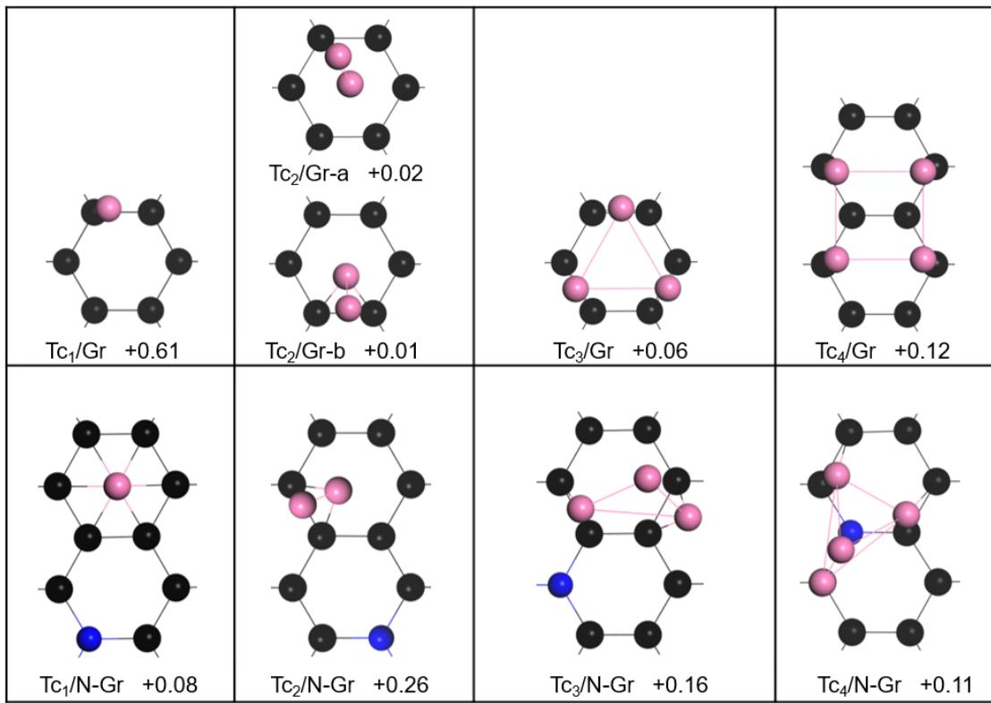
**Figure S7.** The sub-stable structures of Tc<sub>n</sub> (n=1–4) adsorption on Gr and N-Gr surfaces
