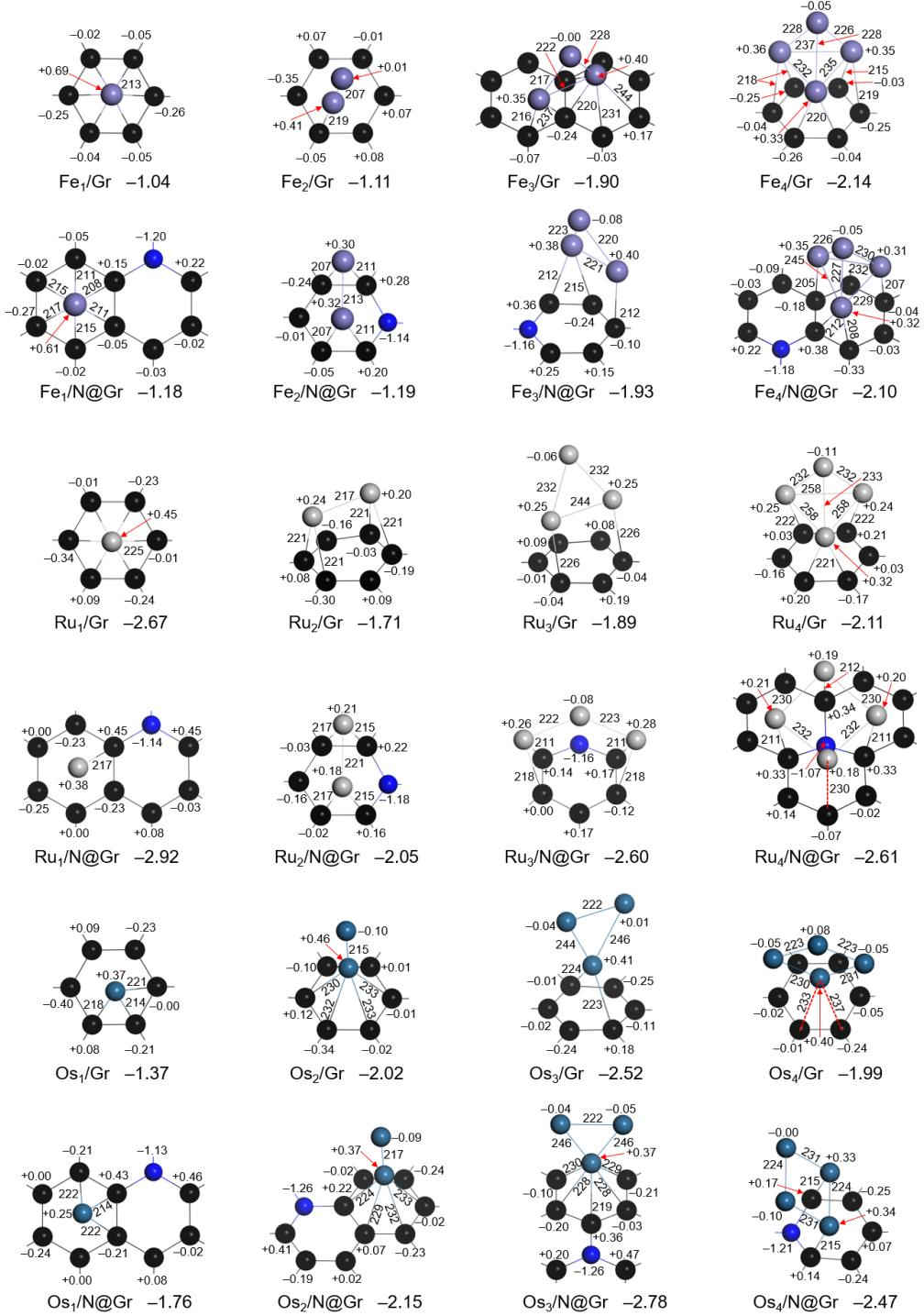
**Figure S2.** Bond lengths (pm),  $E_{\text{ads}}$  (eV), and Bader charges ( $e$ ) for the most stable configuration of  $\text{TM}_n$  clusters ( $\text{TM} = \text{Fe}, \text{Ru}$  and  $\text{Os}$ ;  $n = 1\text{--}4$ ) adsorption on Gr and N-Gr surfaces. Fe, Ru and Os atoms are shown in purple, grey, and deep green balls, respectively.
