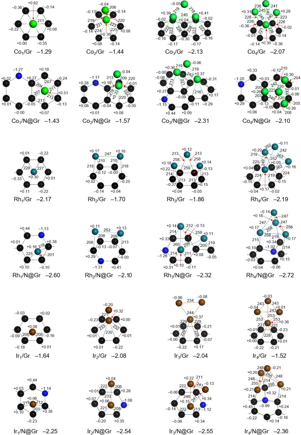
**Figure S3.** Bond lengths (pm),  $E_{\text{ads}}$  (eV), and Bader charges ( $e$ ) for the most stable configurations of  $\text{TM}_n$  clusters ( $\text{TM} = \text{Co, Rh and Ir}; n = 1\text{--}4$ ) adsorption on Gr and N-Gr surfaces. Co, Rh and Ir atoms are shown in light green, deep green, and brown balls, respectively.
