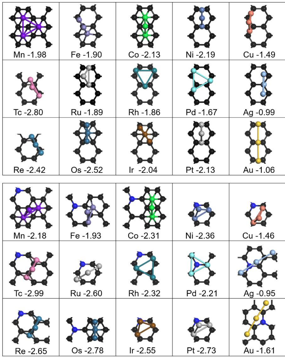
**Figure S22.** Summary for the adsorption of TM trimers on Gr (the top) and N-Gr (the bottom) surfaces with associated  $E_{\text{ads}}$  (eV).
