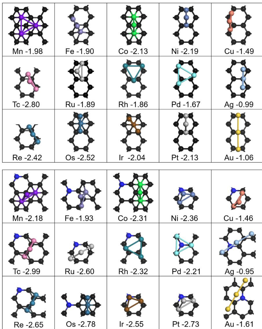
**Figure S23.** Summary for the adsorption of TM tetramers on Gr (the top) and N-Gr (the bottom) surfaces with associated  $E_{\text{ads}}$  (eV).
