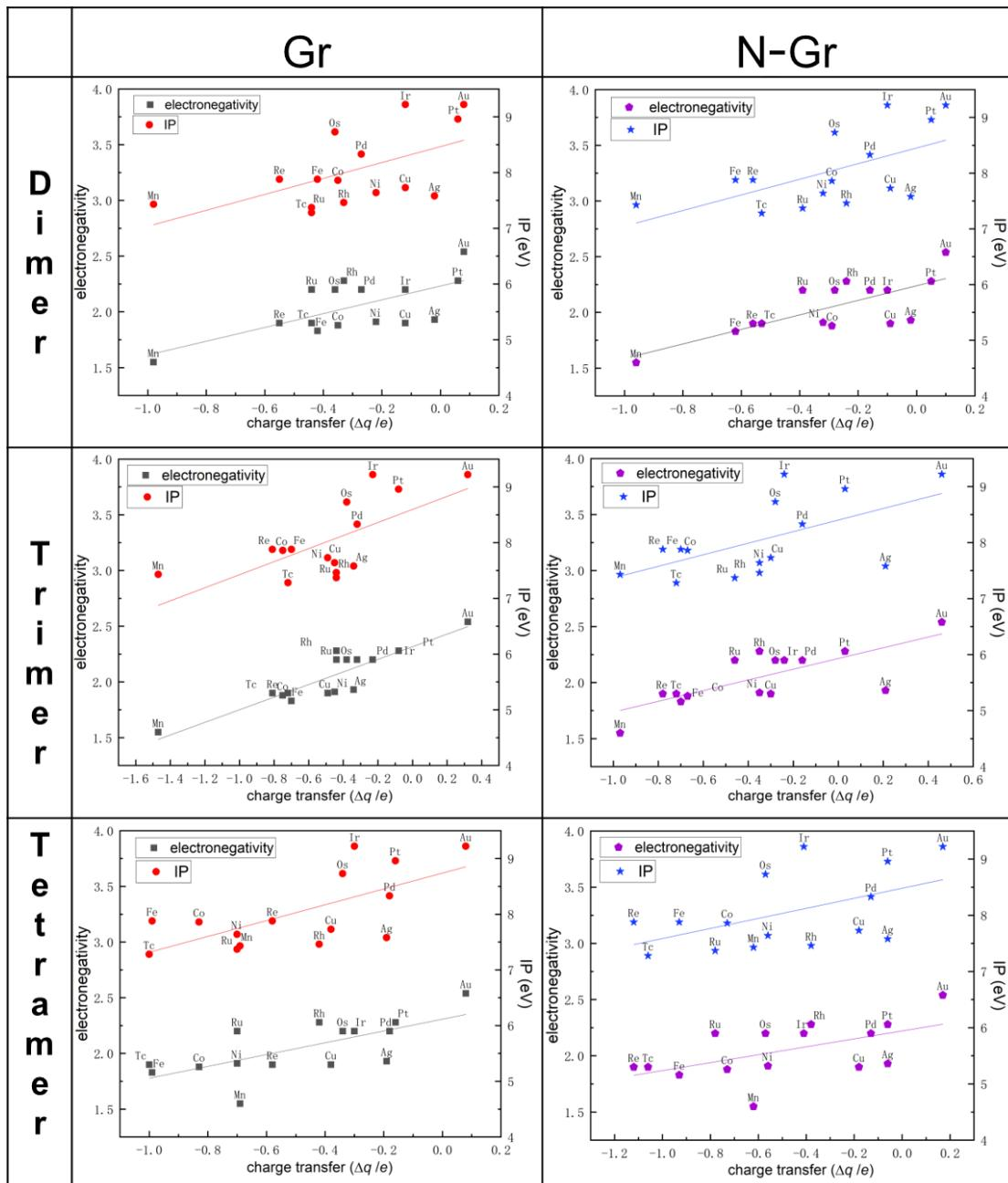
**Figure S25.** Plots of electronegativity and IP versus charge transfer for dimers, trimers, and tetramers on Gr (the left) and N-Gr (the right) surfaces.
