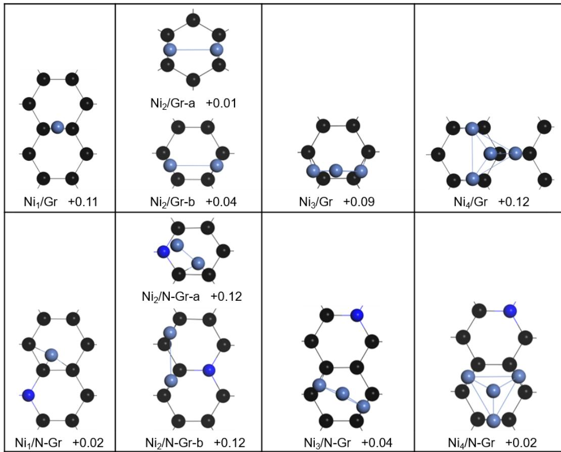
**Figure S15.** The sub-stable structures of Ni<sub>n</sub> (n=1–4) adsorption on Gr and N-Gr surfaces with relative energies  $\Delta E$  (eV).
