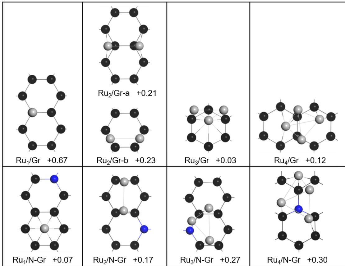
**Figure S10.** The sub-stable structures of Ru<sub>n</sub> (n=1–4) adsorption on Gr and N-Gr surfaces with relative energies  $\Delta E$  (eV).
