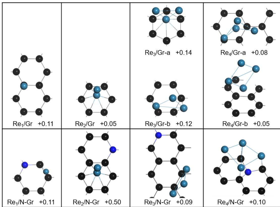
**Figure S8.** The sub-stable structures of Re<sub>n</sub> (n=1–4) adsorption on Gr and N-Gr surfaces with relative energies  $\Delta E$  (eV).
