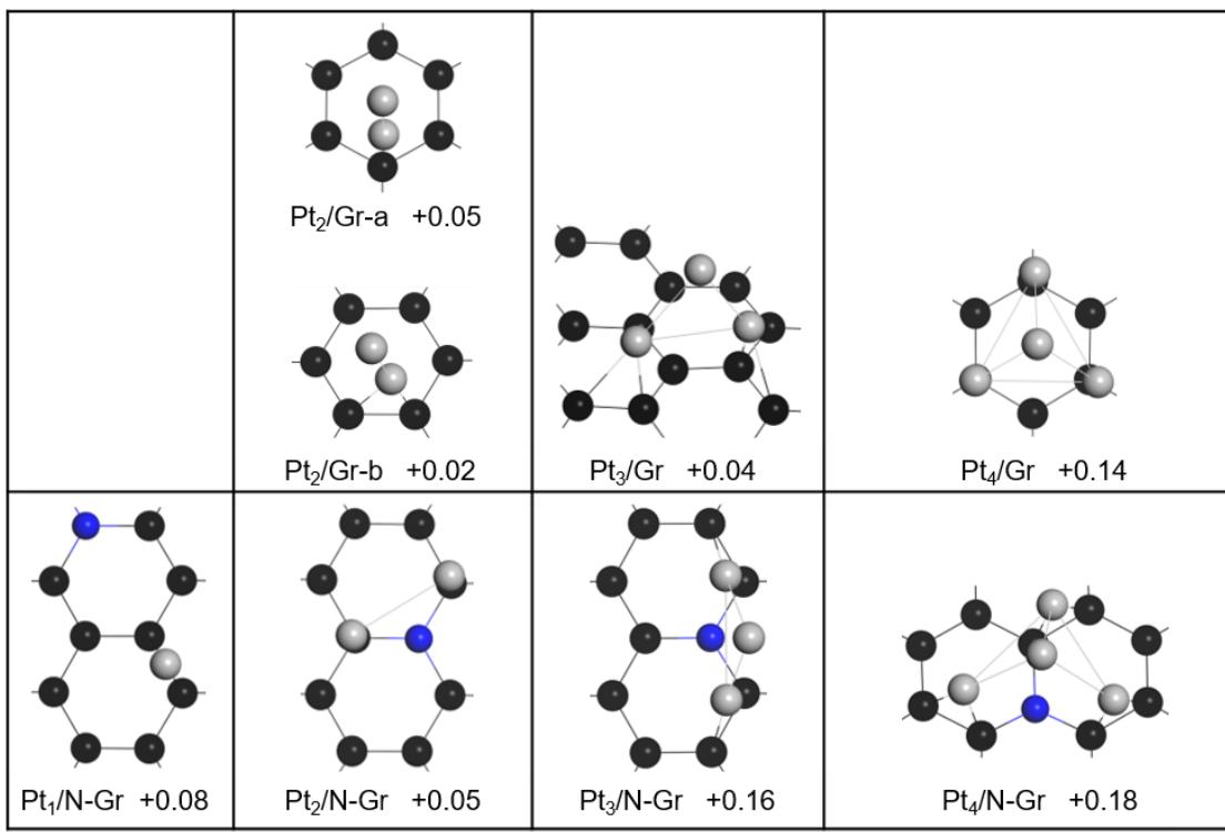
**Figure S17.** The sub-stable structures of Pt<sub>n</sub> (n=1–4) adsorption on Gr and N-Gr surfaces with relative energies  $\Delta E$  (eV).
