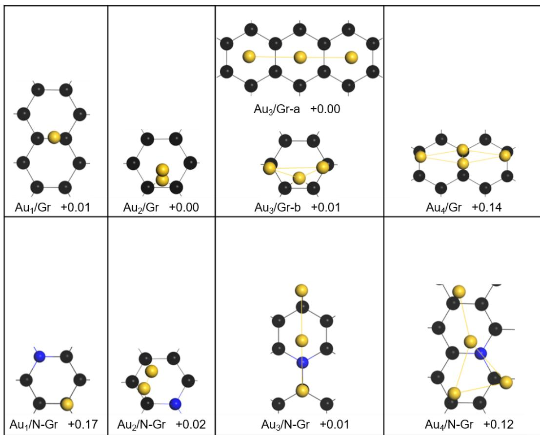
**Figure S20.** The sub-stable structures of Au<sub>n</sub> (n=1–4) adsorption on Gr and N-Gr surfaces with relative energies  $\Delta E$  (eV).
