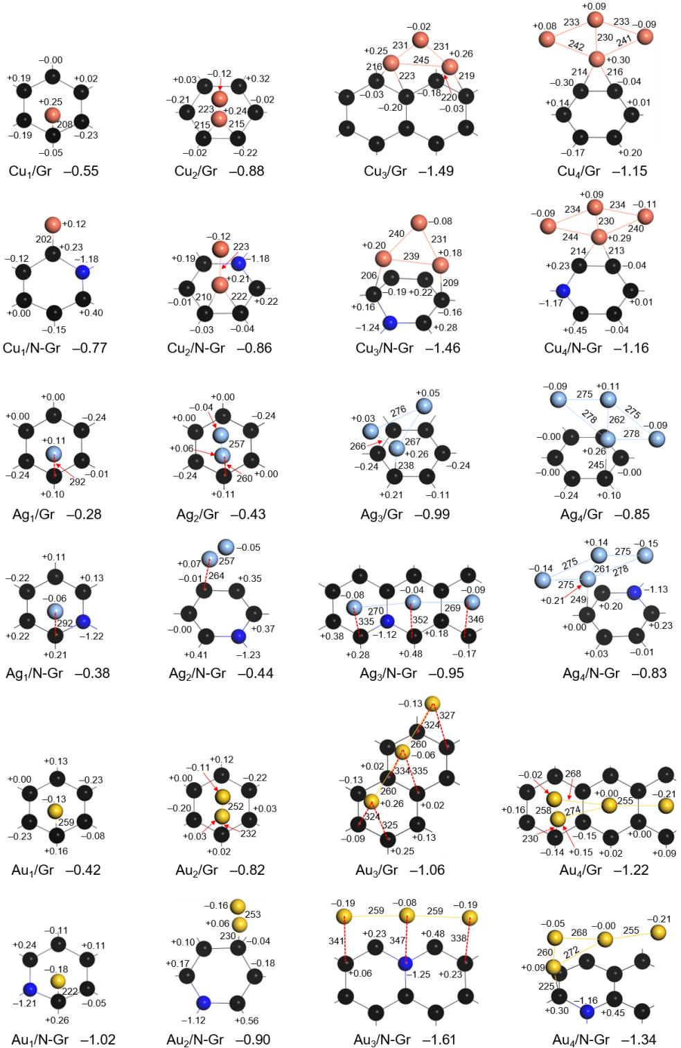
**Figure S5.** Bond lengths (pm),  $E_{\text{ads}}$  (eV), and Bader charges ( $e$ ) for the most stable configurations of  $\text{TM}_n$  clusters ( $\text{TM} = \text{Cu}, \text{Ag}$  and  $\text{Au}$ ;  $n = 1–4$ ) adsorption on Gr and N-Gr surfaces. Cu, Ag and Au atoms are shown in copper, light blue, and gold balls, respectively.
