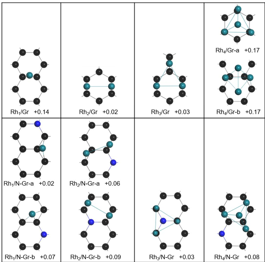
**Figure S13.** The sub-stable structures of Rh<sub>n</sub> (n=1–4) adsorption on Gr and N-Gr surfaces with relative energies  $\Delta E$  (eV).
