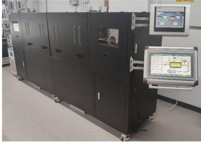
**Figure S2.** Optical photograph of our self-developed batch production CVD equipment for GGF.
