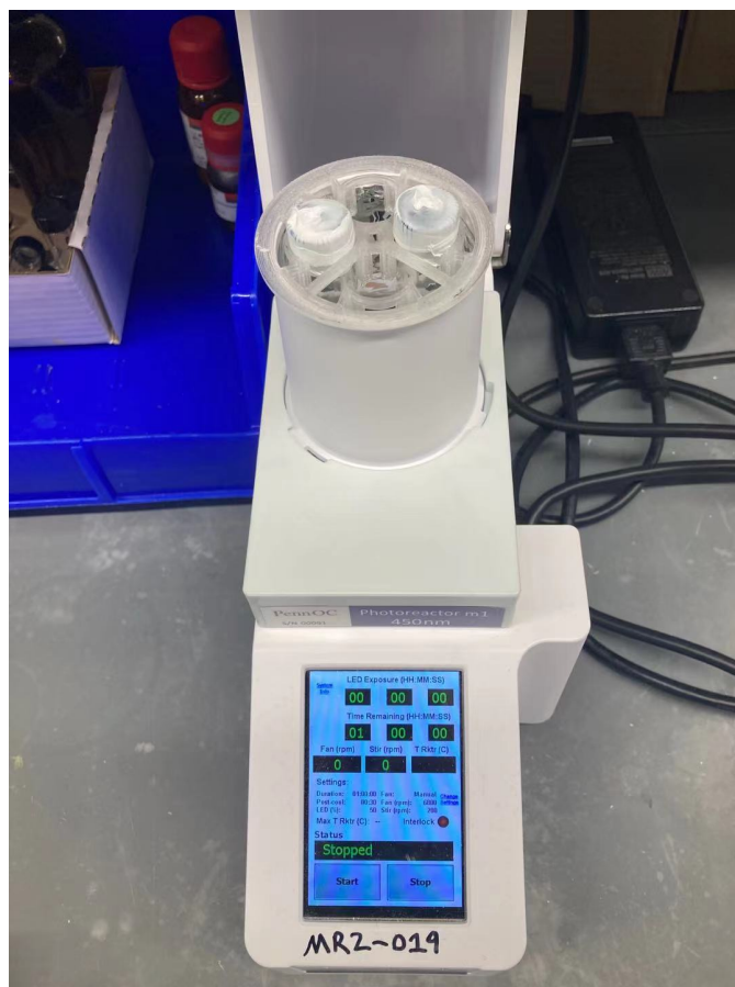
Figure S8. Reaction setup with the Integrated Photoreactor
