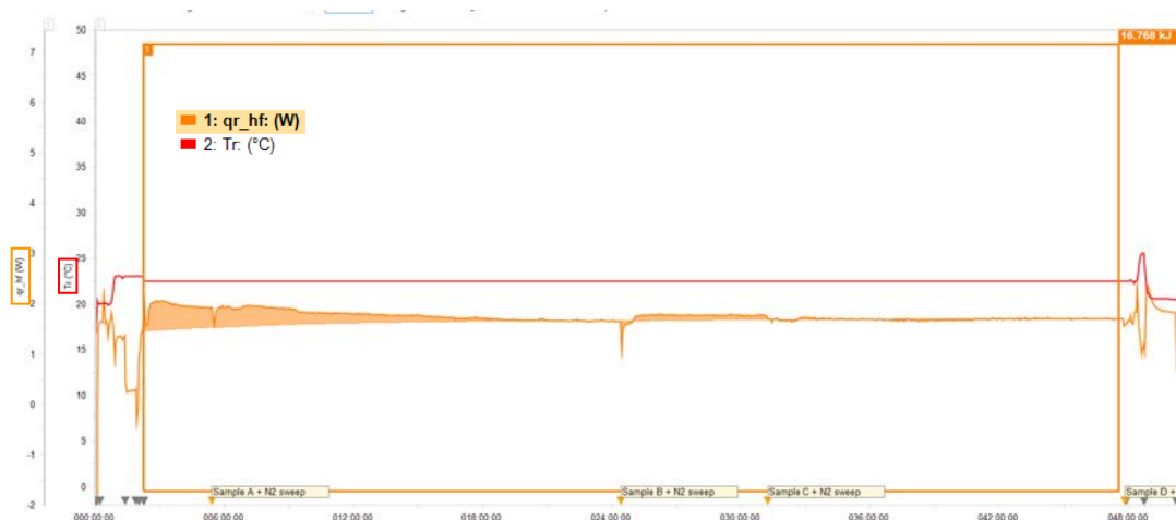
Figure S8: Thermogram for the enantioselective fluorination of 200 g of rac - 1 with CsF under HB-PTC. Red: Temperature inside the reactor; orange: heat flow due to the reaction.
