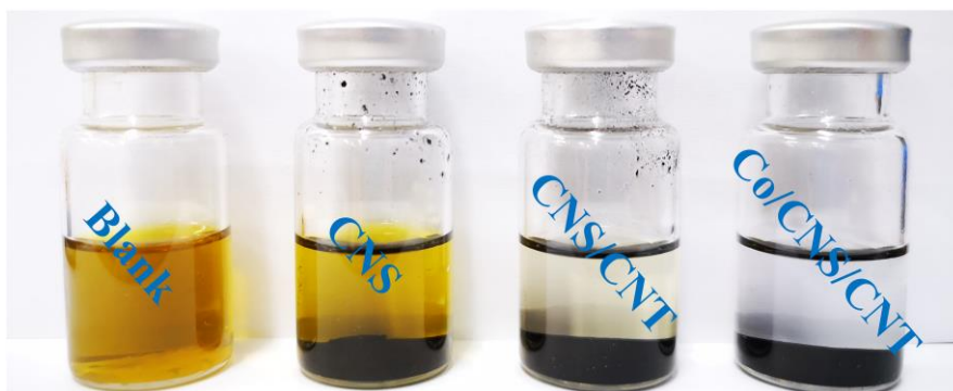
Figure S8. Co/CNS/CNT, CNS/CNT, CNS adsorption capacity test in mixed 5mL DME/DOL solutions of 2 mM \text{Li}_2\text{S}_6 solution.
