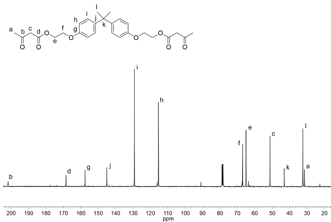
Figure S32. ^{13}\text{C} NMR Spectrum of Bisphenol A diethyl ether acetoacetate (BPAE-A) (100 MHz, \text{CDCl}_3 , 77 ppm)
