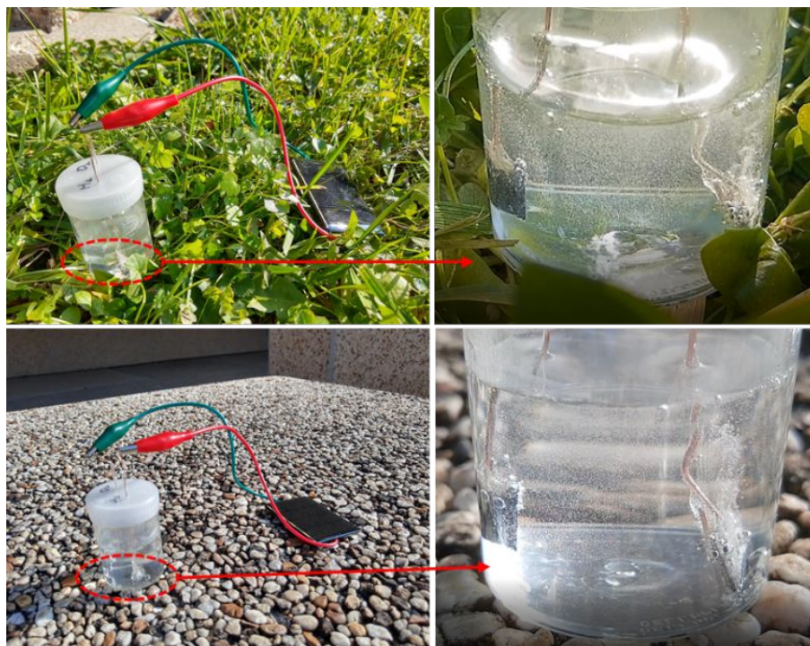
Figure S19. Outdoor Solar light powered overall water splitting for hydrogen and oxygen evolutions.
