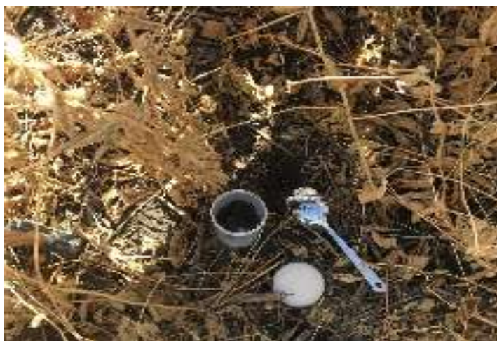
Figure S6. Demonstration of soil sampling using (A) the 12.7 cm metal pipe, and (B and C) soil sample collection in 500-mL polypropylene jars. The soil type of the field is Colo silt loam 12 .
