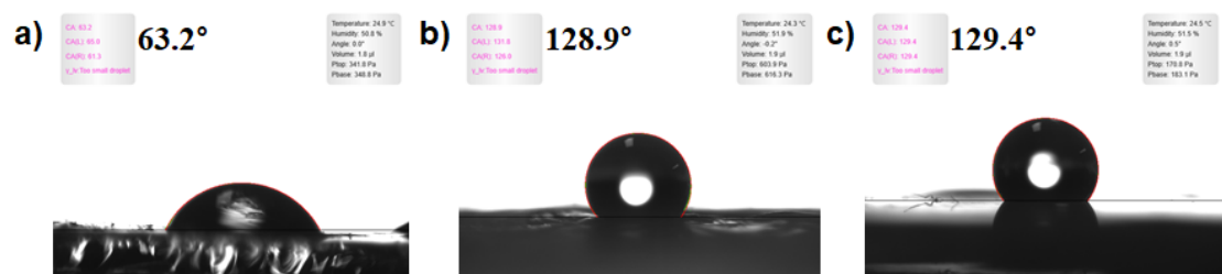
Figure S4. Measured value of water contact angle by substrate a) glass, b) plastic, and c) SMS filter.
