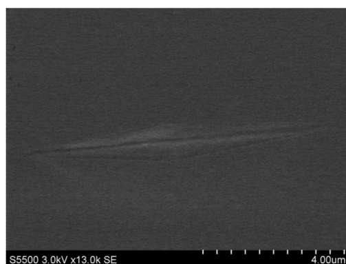
Figure S5 SEM image of an indent made on a Si substrate by a Knoop indenter with a load of 49 mN.
