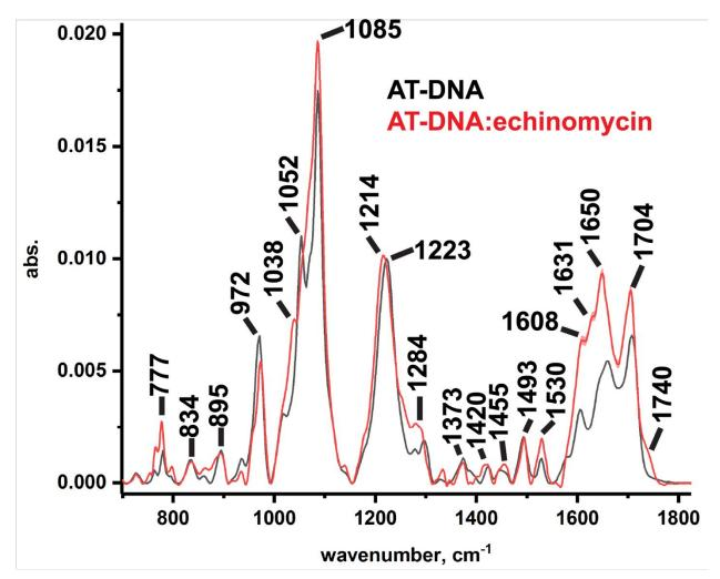
**Supporting Figure 2:** Full IR spectra for AT-DNA when free (black) and when bound to echinomycin (red) showing the characteristic changes upon drug binding. Mean in of three replicates in bold and standard deviation in shade.
