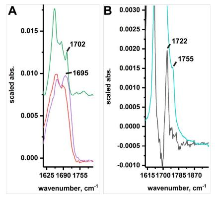
**Supporting Figure 5:** Carbonyl region for (A) single stranded 12-mer of poly-T (red) and N1methylthymine (purple) in water and the A-T Hoogsteen dimer crystal (green) and (B) N1methylthymine in d6-DMSO (cyan) and DMF (black).
