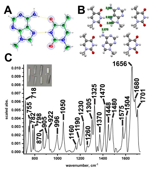
**Supporting Figure 6:** (A) The observed density map for crystals of the N9-methyladenine and N1-methylthymine Hoogsteen dimer. (B) Crystal packing of the dimer showing interactions of the C2=O with atoms in neighboring unit cells. (C) IR spectrum collected from the Hoogsteen dimer crystals (shown in inset). Distances are in angstroms.
