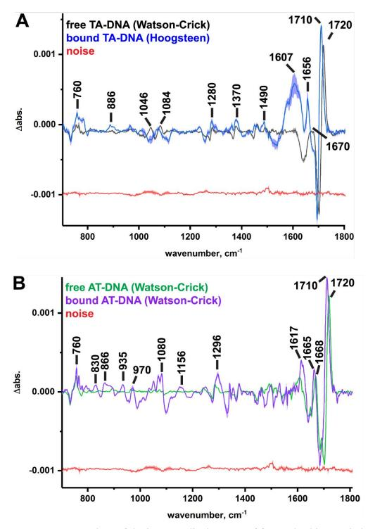
**Supporting Figure 3:** Overlays of the isotope edited spectra of free and echinomycin bound (A) TA-DNA and (B) AT-DNA and a representative noise line (replicate minus replicate for the free TA-DNA).
