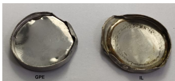
Figure S11. Digital photos of the disassembled coin cell shells of the Al//GPE//Graphite battery and the Al//IL//graphite battery after cycling.
