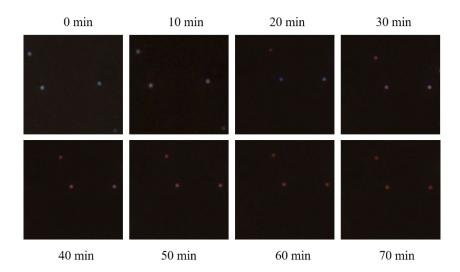
Fig.S6 Dark-field images of Au-Ag-HM nanoprobe incubated with 10  $\mu$ M of H<sub>2</sub>O<sub>2</sub> for different time.
