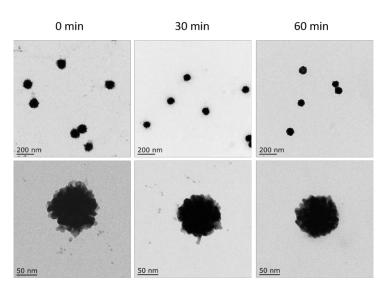
Fig.S5 TEM images of Au-Ag-HM nanoprobe incubated with 10  $\mu M$  of  $H_2O_2$  for
