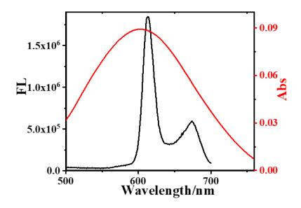
Fig.S4 Fluorescence spectrum of HMME and UV spectrum of AuNFs.
