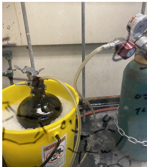
SI-Figure 1: Ammonia gas is bubbled into a cooled 4L of MeOH.
