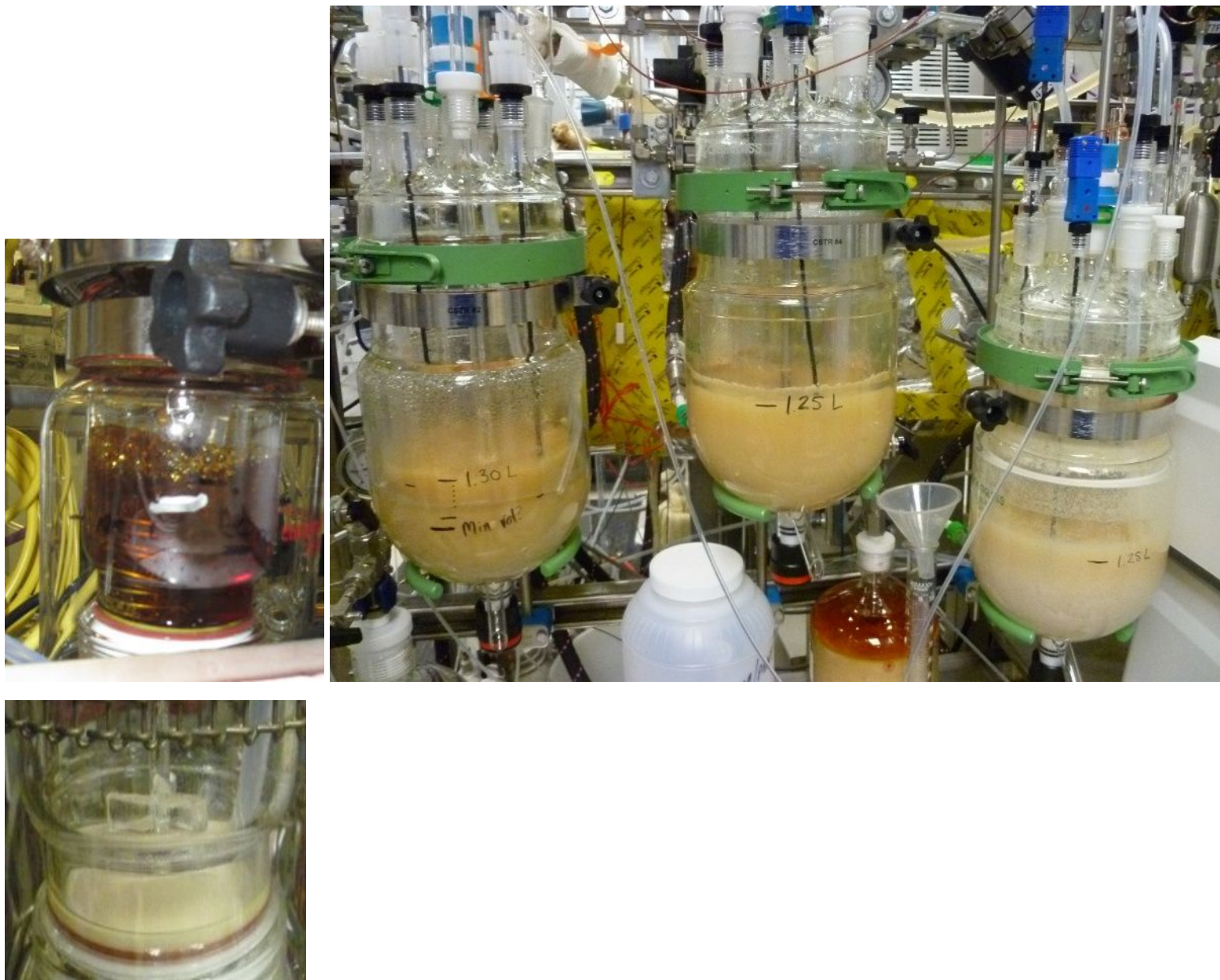
Figure S5. Picture of the 250 mL continuous evaporator, three 2 L MSMPRs, and one of the dual slurry-off filters while running at steady state.
