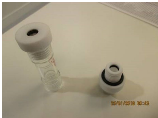
Figure S11. Filter agitator seals used at the beginning of the campaign. These are the O-rings that shed, getting black specks into the product, leading to the reprocessing.
