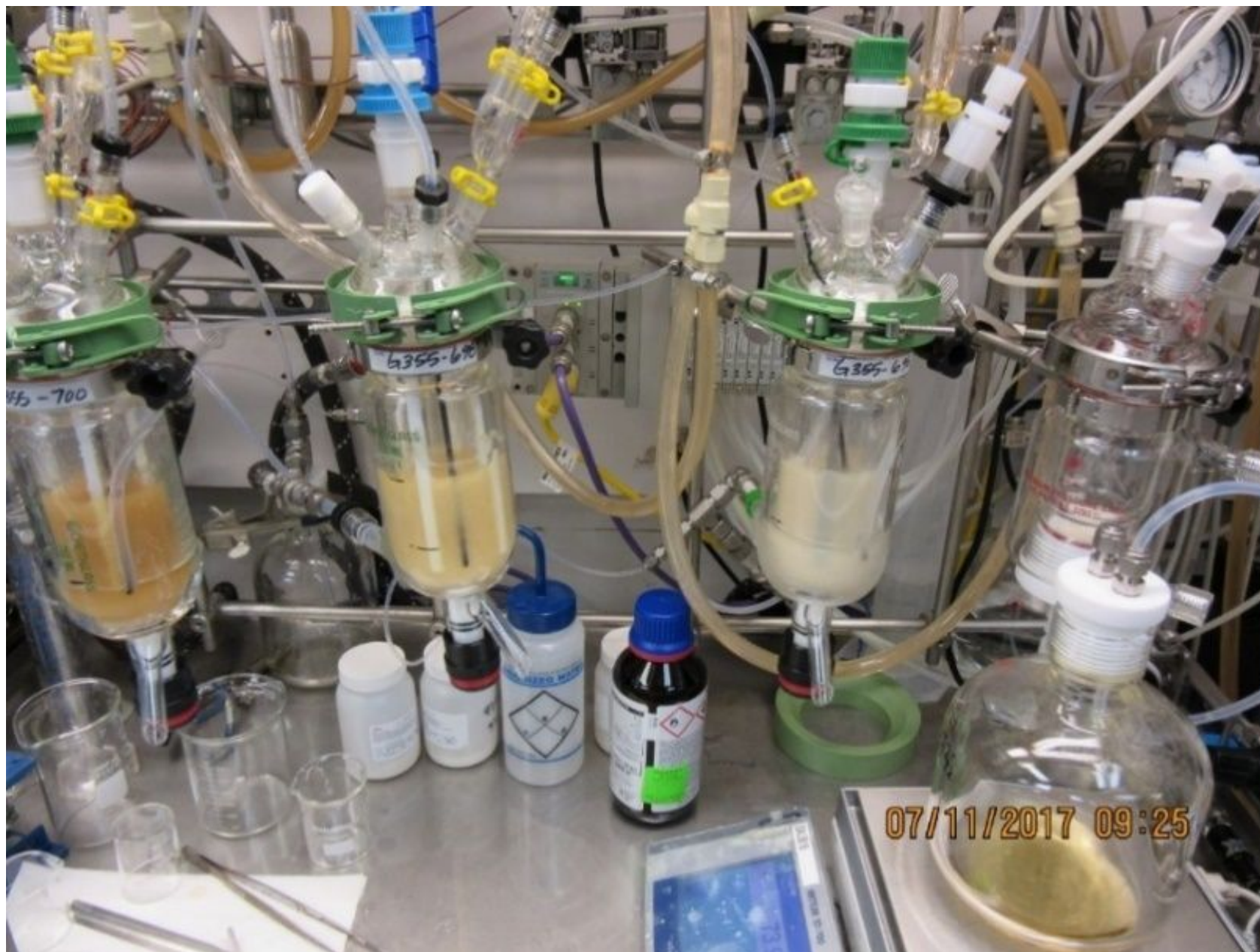
Figure S3. Picture of the 3 MSMPRs in series operating at research scale, MSMPR1, 2 and 3 from left to right.
