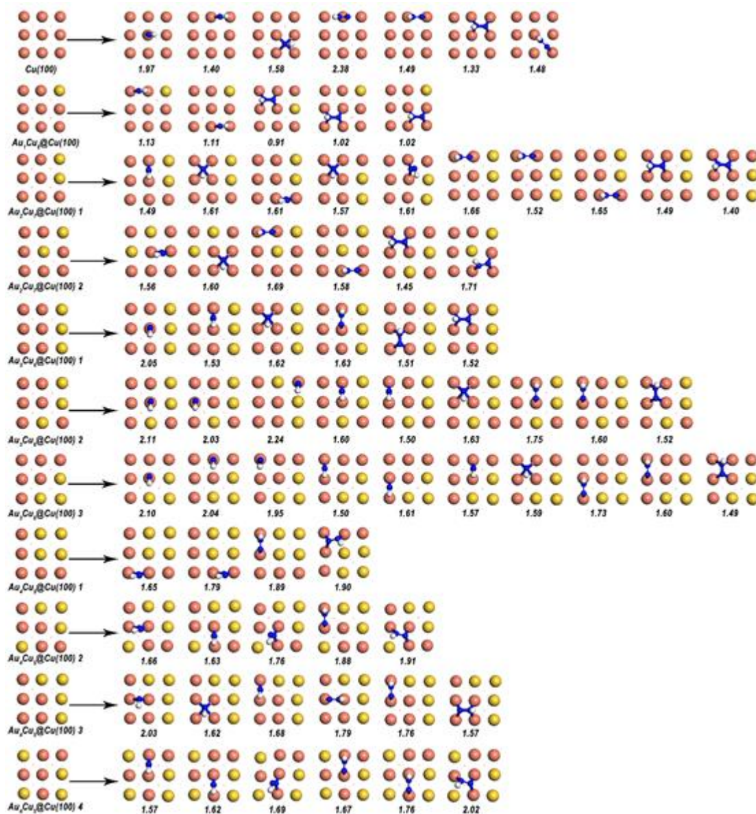
Figure S16. *NNH adsorption configurations considered for \text{Au}_n\text{Cu}_{(9-n)}@Cu(100) with n = 0 to 4.
