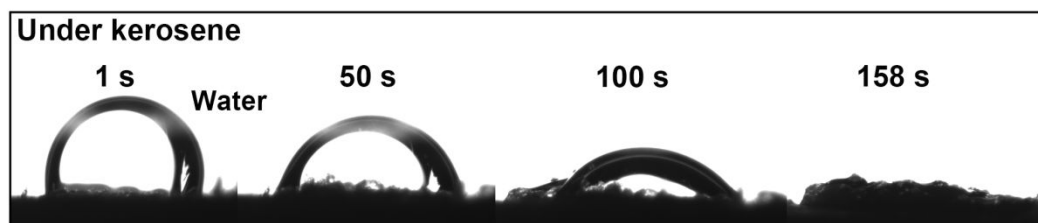
Figure S14 Images of water contact angle showing the permeation of water droplet into collagen fibers under kerosene.
