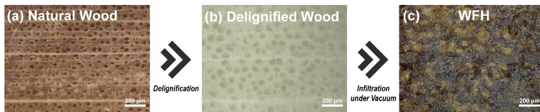
Figure S4. Optical images of different wood during this process. The surface morphologies of (a) natural beech wood, (b) completely delignified wood, and (c) WFH. During this treatment process, the pores of natural wood are opened and filled.
