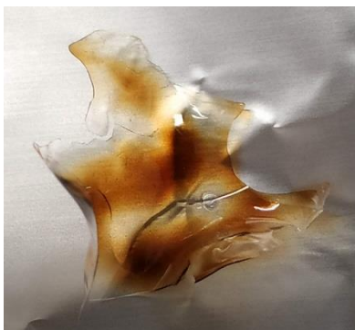
Figure S3. Film representative of the degradation's heterogeneity. CDA acid catalyzed degradation experiment, week 16.
