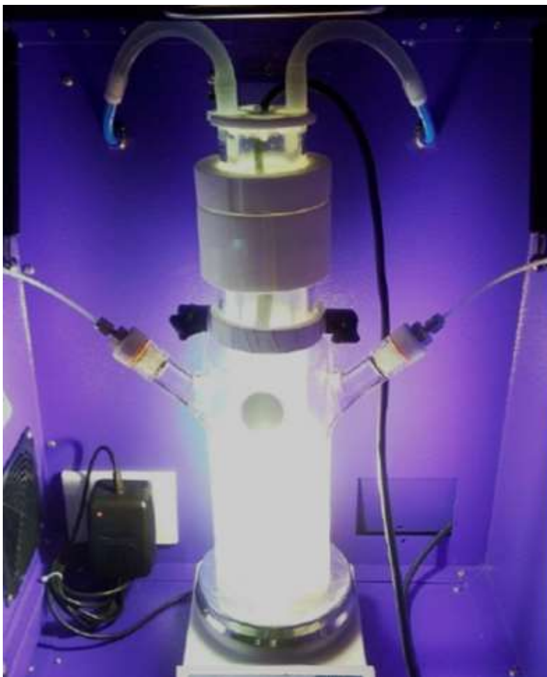
Figure S10. Picture of the employed photo-reactor for photoreduction of \text{CO}_2 to \text{CH}_4 .
