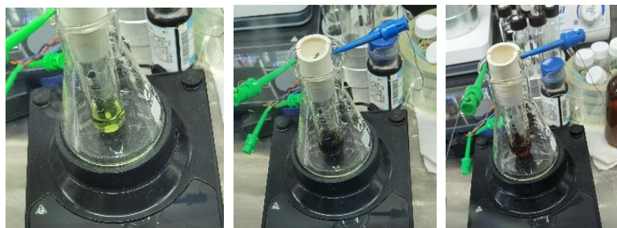
Figure S4. From left to right: (1) Starting the reaction on an electrochemical equipment with a constant current of 4 mA (10 mm electrodes were immersed into the reaction solution); (2) After 2 min stirring, the reaction mixture turned black; (3) After 10 h stirring.
