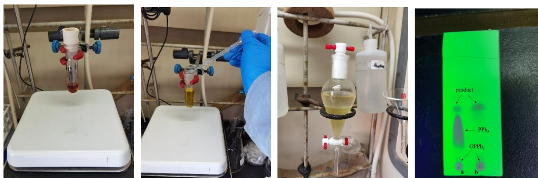
Figure S5. From left to right: (1) The reaction mixture; (2) Diluted with EtOAc (adding the aq. H 2 O 2 was optional); (3) Extraction.; (4) TLC: Lane a : the reaction mixture; Lane b : the reaction mixture after treatment with H 2 O 2 .
