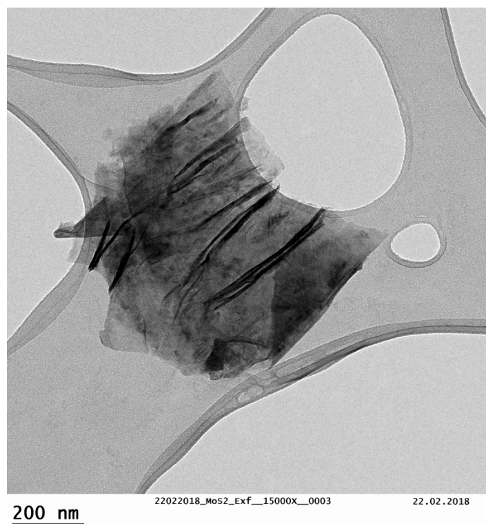
Fig. S2. Representative TEM image of Exf-MoS 2 with an average lateral dimension of 567 \pm 239 nm (Max value: 959 nm, min value: 323 nm) calculated from 10 different measurements.
