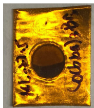
Figure S32. Example EXAFS sample cell using aluminum sheet and Kapton windows. The sample is in supercooled liquid state after running EXAFS experiments at elevated temperature.
