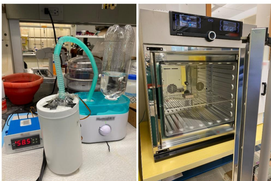
Figure S17. Left: the home-designed humidity chamber which used in the previous work. Right: the humidity oven which used for solid-state hydrolysis in this work.
