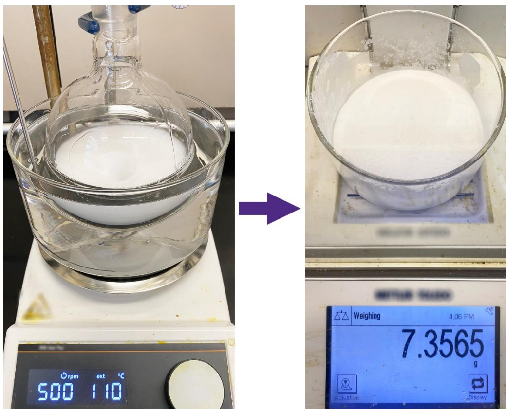
Figure S6. The pictures of water-synthesis of MOF-808-TFA, in which more than 7 grams of activated samples can be obtained from a single reaction at the 150 mL scale.
