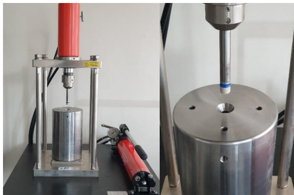
Hydraulic press and high-pressure reactor vessel for high pressure experiments
