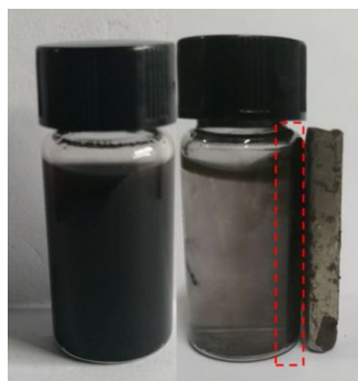
Figure S4. The suspension of 0.15Fe-CoO NCs after ultrasound for 5min (left) and the corresponding state after applying a magnet for 30 min (right).
