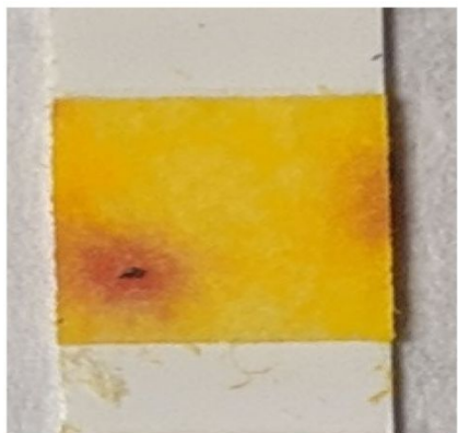
Figure S5. Color change on the tile of a color strip when in contact with a lead solder particle
