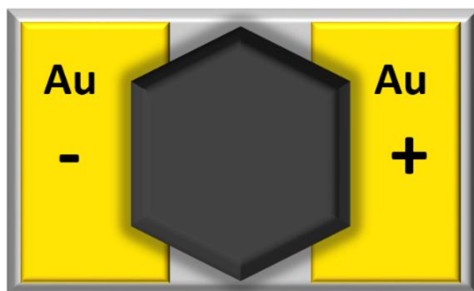
Figure S1. Schematic of laterally structured sample with a \text{CH}_3\text{NH}_3\text{PbI}_3 layer on the top. The test structure consisted of a symmetric 150 nm thick gold electrodes and 45 \mu\text{m} electrode gap distance on a glass substrate.
