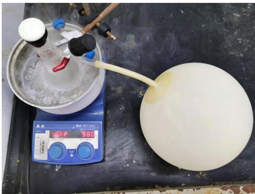
Figure S2 The setup for the synthesis of 1-(diphenylphosphino)-propanone.
