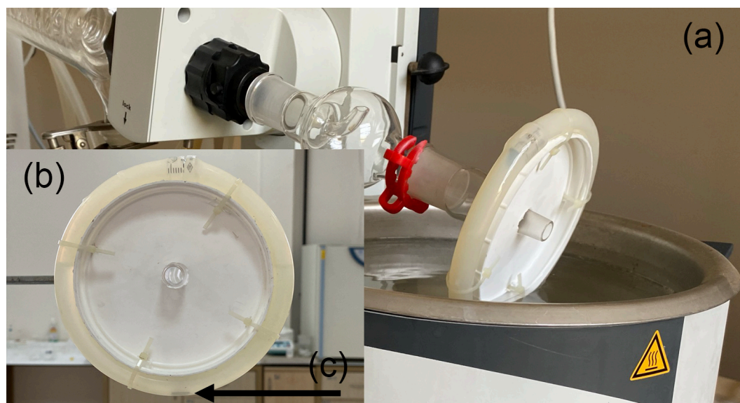
Figure S1. Photographs of the homemade rotary flow system (taken by Dr. Demirci) which was connected evaporator (a), the flow system (b), and PILs grafted silicon wafer (c) in a silicone tube.
