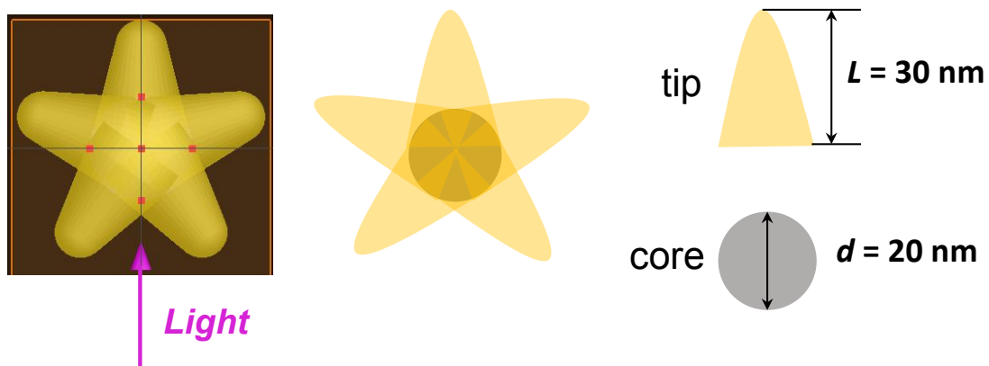
Figure S4. Schematics of the models for theoretical calculations. The core with a diameter of 20 nm surrounding five 30 nm length tips. Since the size of gold and silver seeds all are distributed between 15 and 20 nm, and the final diameters reach 50-60nm. Consequently, the nanostars were assumed into two parts: perfect sphere core part with a diameter of 20 nm, and five branches parts with 30 nm length and not sharp tip with a diameter of 10 nm evenly distributed on one plane, which was evaluated by TEM results( Figure 3I , Figure 4I ).
