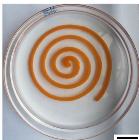
Figure S6. The printed spiral structure after printing for 1 h. The concentrations of CNC and chitosan are 1 wt.% and 0.5 wt.%. The pH of the dextran and PEG aqueous solution are 3.5 and 2.5. The scale bar is 1 cm. Fluorescein sodium with a concentration of 1.2 mg/ml in dextran solution was used to increase the image contrast.
