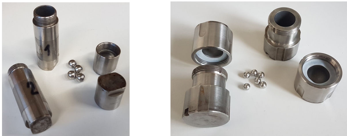
Figure S1. Stainless steel milling vessels used in mechanochemical reactions; left: 5 mL, right: 10 mL.
