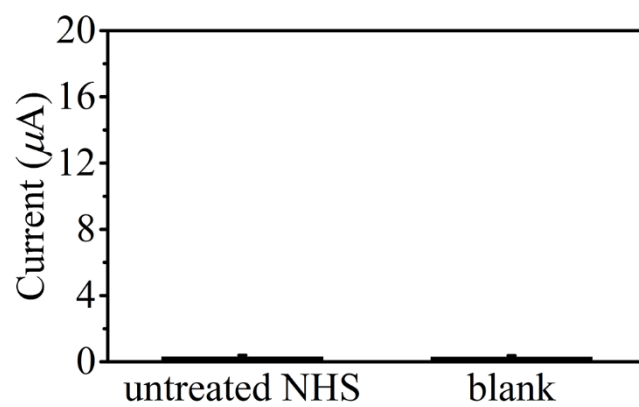
Figure S-6: Peak currents derived from the untreated NHS and the blank control. Error bars show the standard deviations ( n = 4 ).
