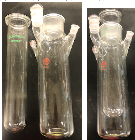
Figure S1. Experimental set-up for low temperature photolyses.
