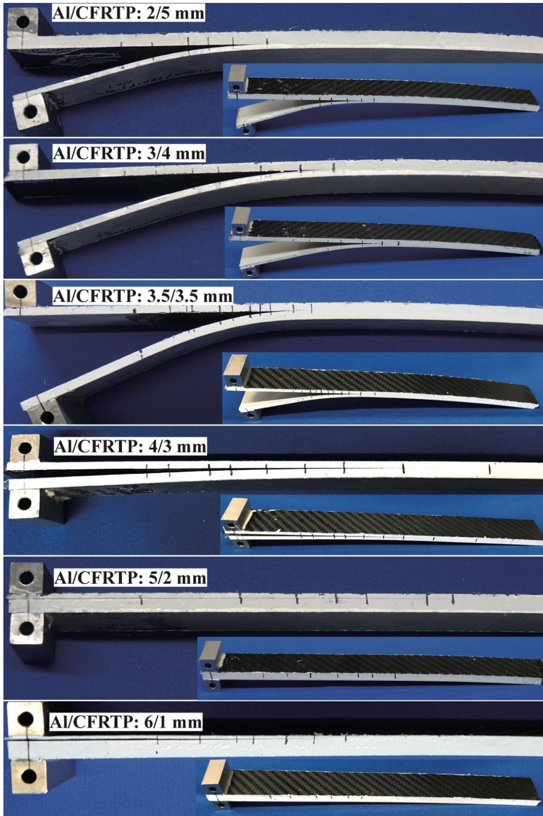
Figure. S2 Al/CFRTP thickness ratio dependence on the plastic deformation of the Al beams after the DCB test of the Al/CFRTP adhesive joints. The total thickness was fixed at 7mm and the thickness ratio was varied.
