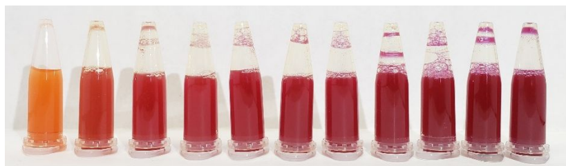
(a) Visualized color changing with \text{Al}_2\text{O}_3 nanoparticles concentration (0 to 0.1 wt.%)
